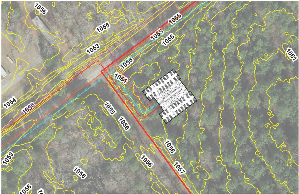
Figure 10. Utility layout with route to first building.
