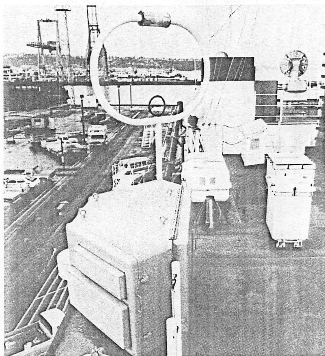
AN/SLQ-32 Electronics Warfare System Antenna. The AN/SLQ-32 is designed to detect, track, and identify contacts by analysis and classification of radar signals.
