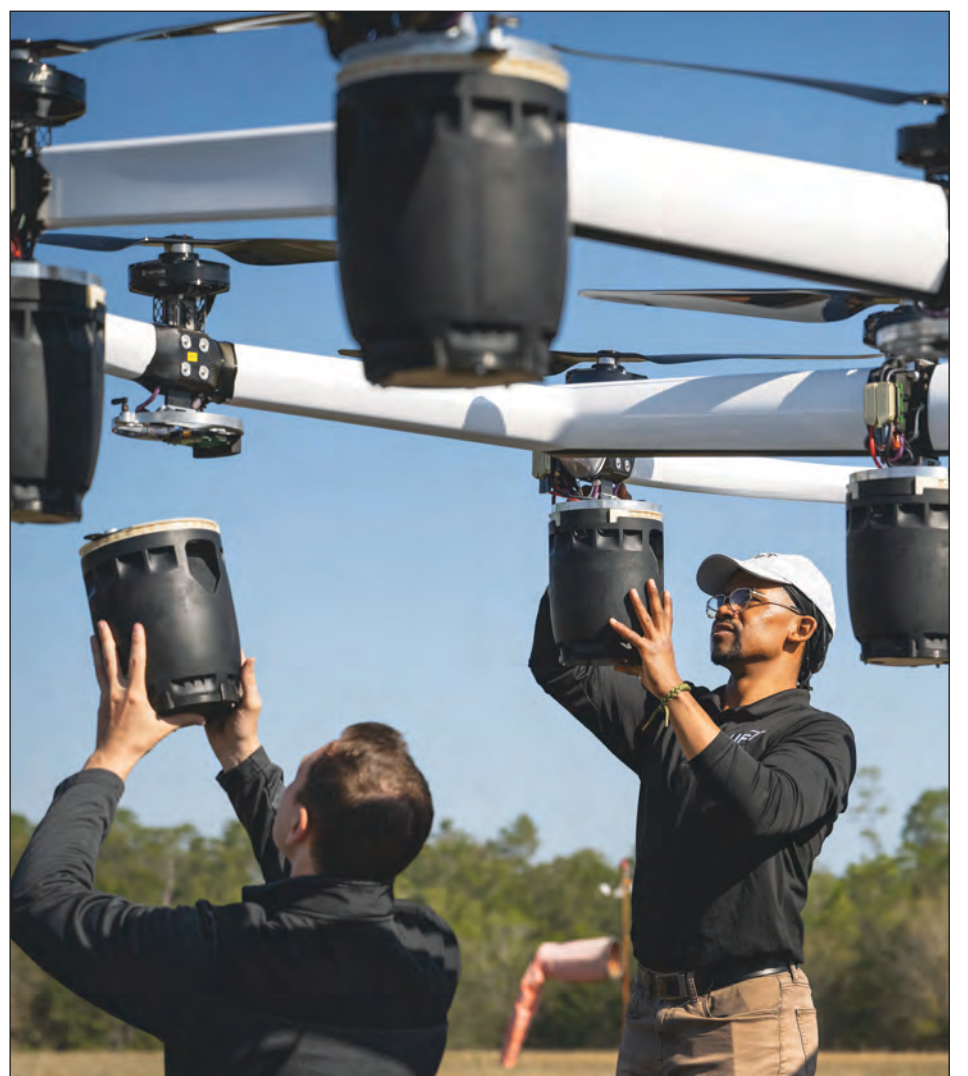
A LIFT team member secures a battery to one of the Hexa’s motors before its first flight April 4 at Eglin Air Force Base, Fla. The Hexa team completed the aircraft’s first unmanned flight test via remote control. The aircraft, which used 18 motors and propellers, flew for approximately 10 minutes and reached a height of about 50 feet. (U.S. Air Force photo by Samuel King Jr.)
