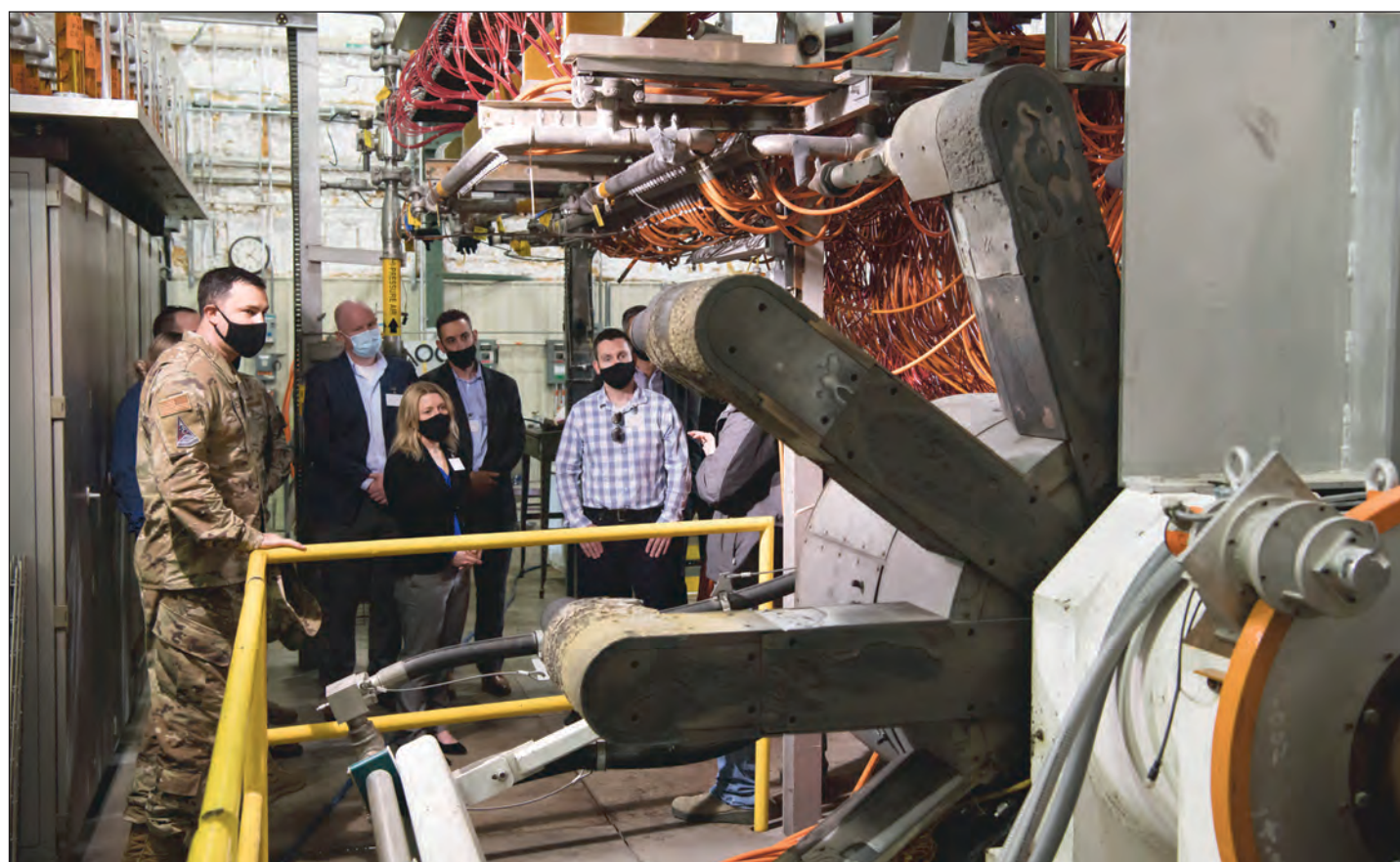
Air Force and defense industry representatives involved in the Ground Based Strategic Deterrent program tour one of the arc jet test cells at Arnold Air Force Base, April 29, 2021. Arnold Engineering Development Complex, headquartered at Arnold AFB, is preparing to support the GBSD program across the complex. The arc heater facilities will be used to study thermal protection systems. (U.S. Air Force photo by Jill Pickett) (This image has been altered by obscuring badges for security purposes.)
