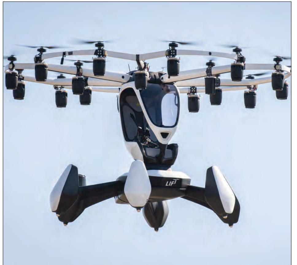
The Hexa, an electric, vertical takeoff and landing aircraft, hovers in the air during its first test flight April 4 at Eglin Air Force Base, Fla. The Hexa team completed the aircraft’s first unmanned flight test via remote control. The aircraft, which used 18 motors and propellers, flew for approximately 10 minutes and reached a height of about 50 feet. (U.S. Air Force photo by Samuel King Jr.)
