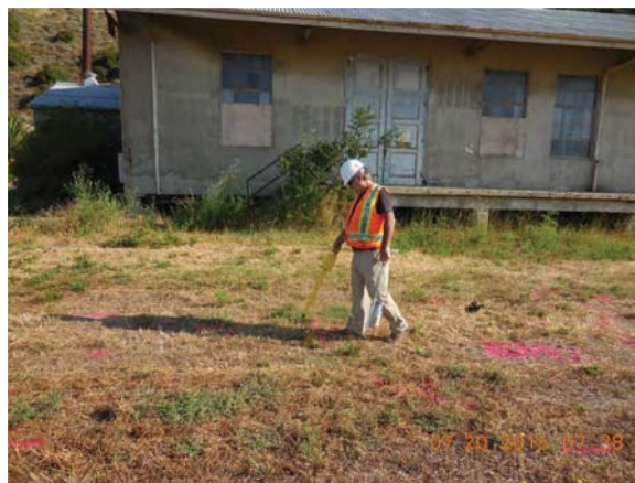
Geophysical survey of Debris Pit in Grid AF011 of SSA using electromagnetic methods
