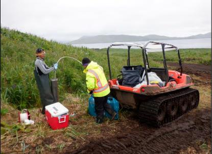
60 monitoring wells were installed to determine the presence of site groundwater and to determine if POL releases had reached groundwater. 47 wells produced sufficient water for successful sample collection.
