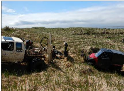
UVOST was used to detect POL in surface and subsurface soils. Soil samples were collected across the site to document contamination across the FUDS.
