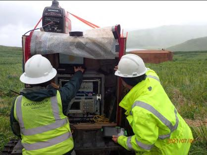
During 2021 field work, UVOST and TarGOST field screening technologies were deployed and were successful in finding subsurface POL plumes in soil.
