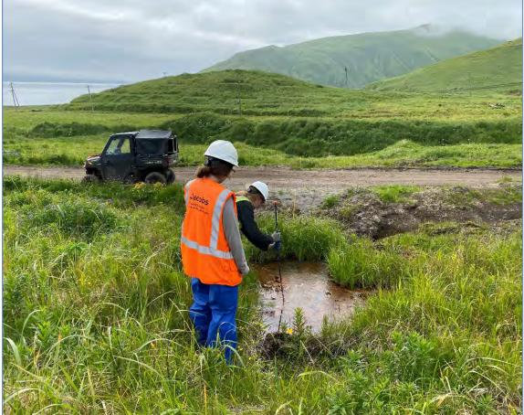
The presence / absence of petroleum sheen was documented for all water bodies found on site. Avalanch probe was used to disturb the sediment to see if sheen could be produced.
