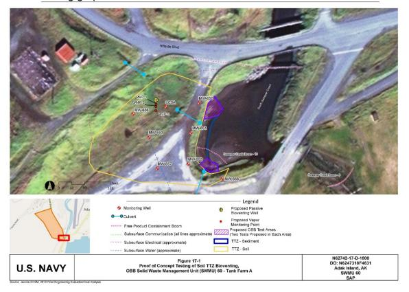
Following the testing period (30-60 days), the collected data were evaluated to determine if wind-assisted passive bioventing and OBB are viable technologies and full-scale remedy design should proceed. The completion of fieldwork in summer 2019 concluded that wind-driven passive bioventing was ineffective. However, the OBB was successful at adsorbing sheen onto the test sections. Thus, design of the OBB portion of the SWMU 60 Remedy Enhancement shall continue.
