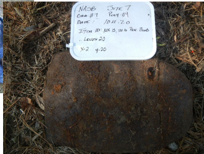
Flattened front half of practice bomb body; several found in the north. No hazard associated with these.
