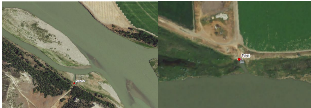
Figure 3-17. Example of Irrigation Intake Located on Side Channel
