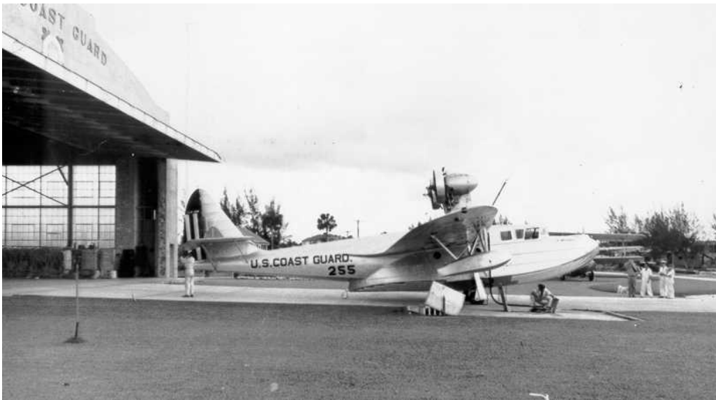
Fokker PJ-1, Coast Guard No. 255, at Air Station Miami. This is the type of seaplane flown by LCDR Leamy on the rescue described in this article. These aircraft were built specifically for the Coast Guard. They were known in the service as FLB's or Flying Life Boats.
