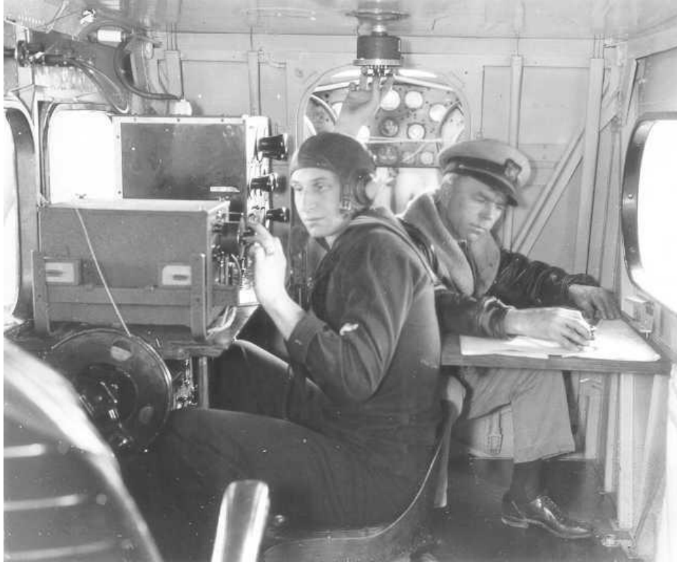
The radio direction finding equipment used to locate vessels in distress as described in this article. Note the operator adjusting the direction-finding antenna on the roof of the cabin as he attempts to locate the direction of an incoming radio signal.
