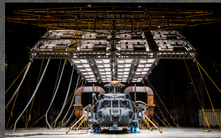
An HH-60W Jolly Green II sits under bright lights used to create heat in the McKinley Climatic Lab March 19 at Eglin Air Force Base, Florida. The Air Force's new combat search and rescue helicopter and crews experienced temperature extremes from 120 to minus 60 degrees Fahrenheit as well as torrential rain during the month of testing. The tests evaluate how the aircraft and its instrumentation, electronics and crew fare under the extreme conditions it will face in the operational Air Force.
