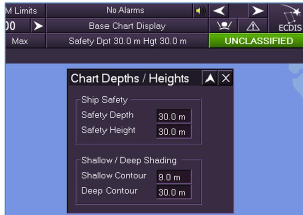
Figure 2-2: Safety Depth display
