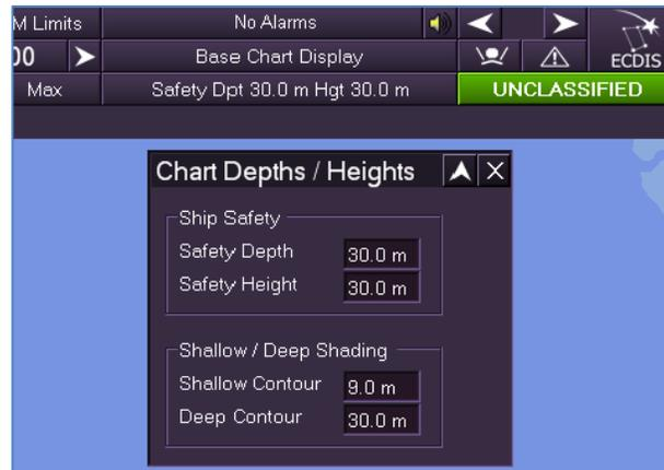
Figure 2-2: Safety Depth display
