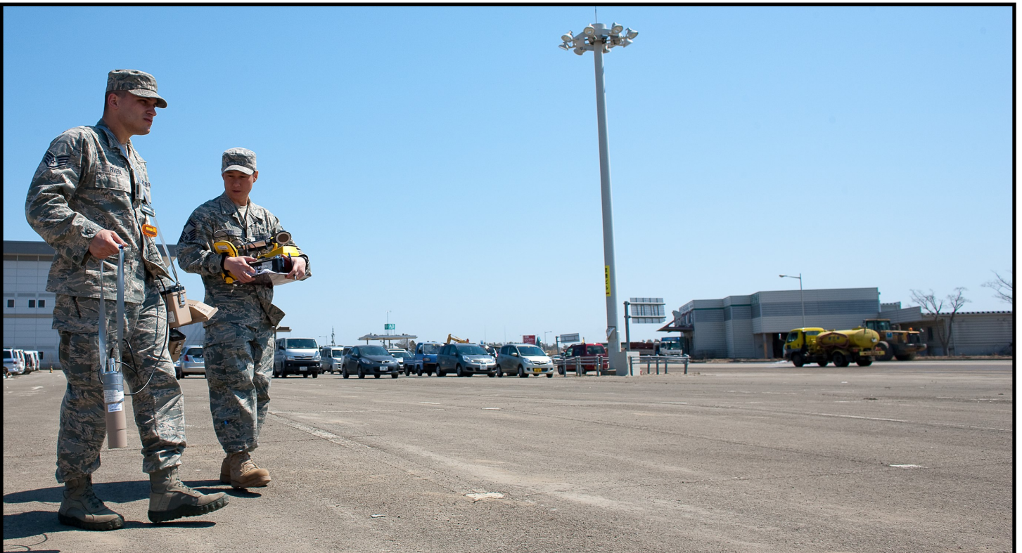
Top: Staff Sgt. Kevin Rivera collects seawater sample at Onahama port, Fukushima Prefecture, 29 March (USAF photo/ Yasuo Osakabe). Bottom: Staff Sgt. Kevin Rivera (left) and Senior Master Sgt. Dean Kim use a sodium iodide detector to check for radiation at Sendai Airport on 5 April 2011. Sergeants Rivera and Kim checked for radiation in the air, soil, and vegetation (USAF photo/Yasuo Osakabe).
