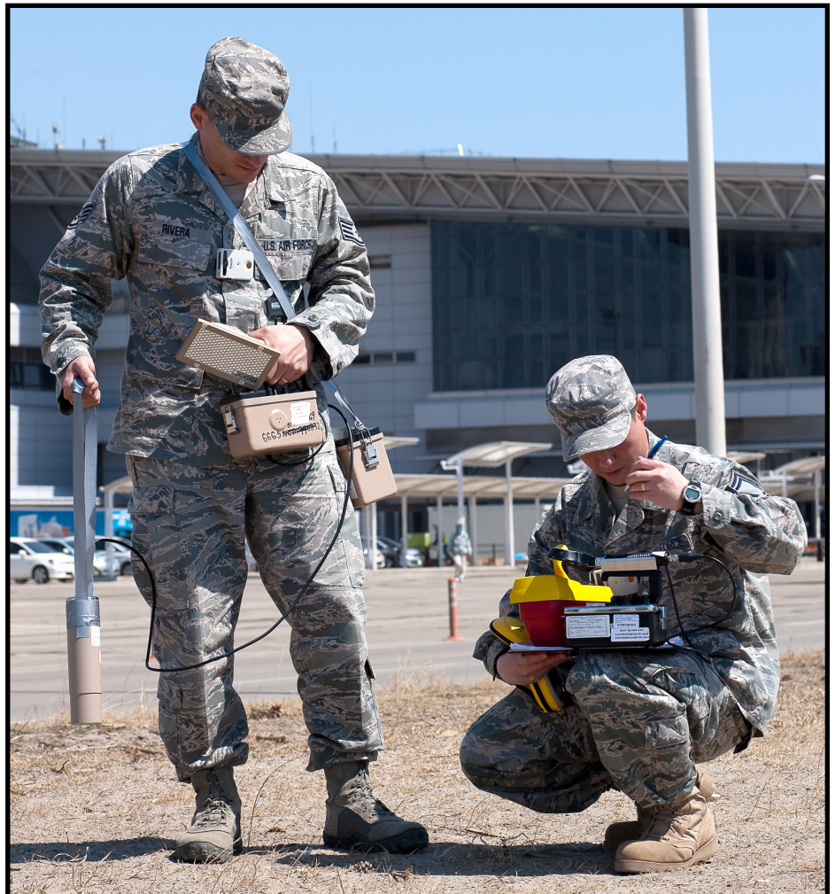
Top: Staff Sgt. Kevin Rivera collects a vegetation sample at Sendai Airport 5 April 2011 (USAF photo/Osakabe Yasuo). Bottom: Staff Sgt. Kevin Rivera (left) and Senior Master Sgt. Dean Kim use a sodium iodide detector to check for radiation at Sendai Airport on 5 April 2011 (USAF photo/Yasuo Osakabe).
