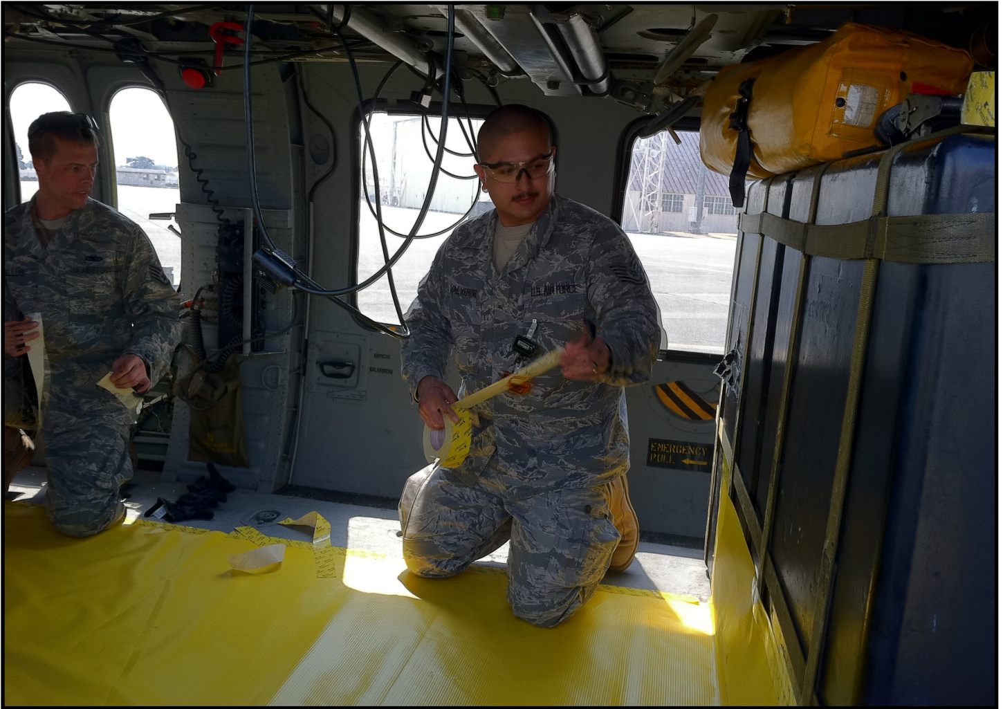
Top: Technical Sgt. Cesar Valverde lines the inside of a HH-60 Pave Hawk for contamination avoidance. TSgt. Valverde also served as AFRAT's expert for radiological instrumentation calibration and repair. Bottom: Master Sgt. Nancy Connell conducts air sampling in base housing with the US Army.
