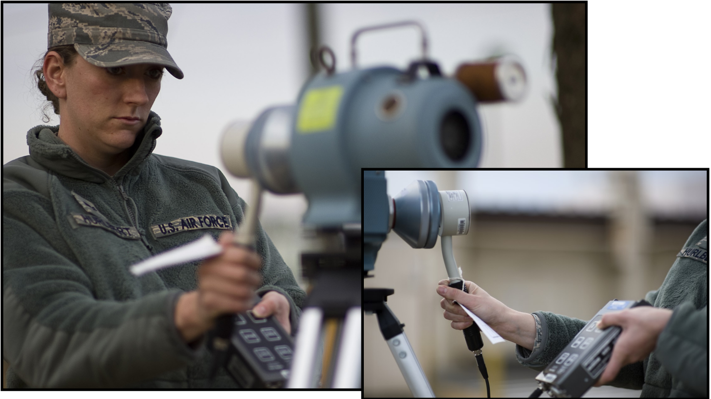
Top: Senior Airman Anna Hurlbert, 18 th Aerospace Medicine Squadron, uses a Radeco to monitor radiation levels in the air at Yokota Air Base, Japan, on 24 March 2011. Airman Hurlbert was on temporary duty from Kadena AB assisting Yokota's Medical Group to monitor base radiation levels in support of Operation TOMODACHI (USAF photo/MSgt Jeremy K. Cross). Bottom: Senior Airman Thompson Kongmany and Senior Airman Mark Williams, 374 th Maintenance Squadron metal technicians, create a camera mount on 28 March 2011. Maintainers were tasked to create a mount for equipment that would monitor radiation levels near reactors at the Fukushima nuclear plant (USAF photo/A1C Andrea Salazar).
