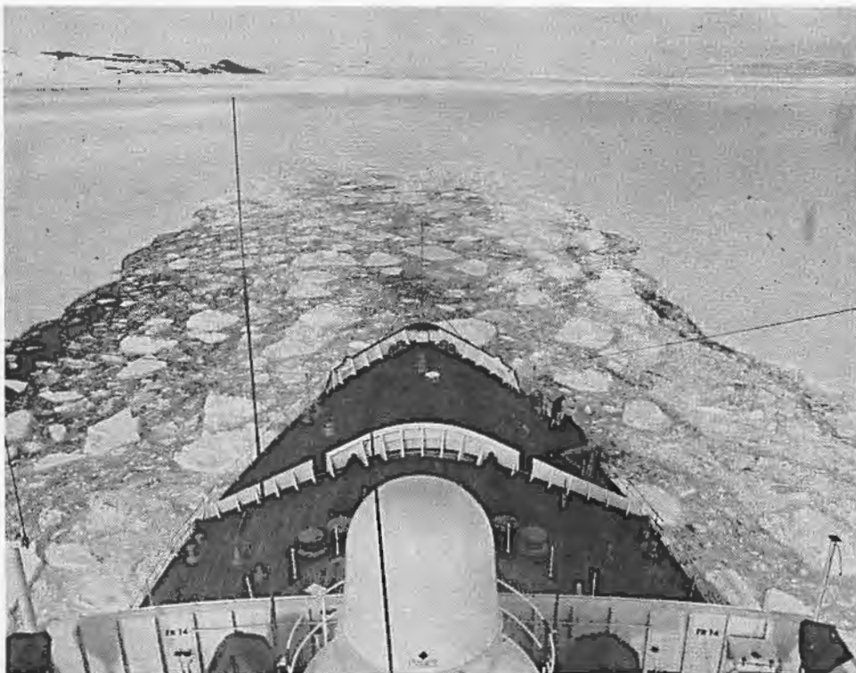
Plate 3. Channel break in, going ahead for another ram. Hut Point in background on left.
