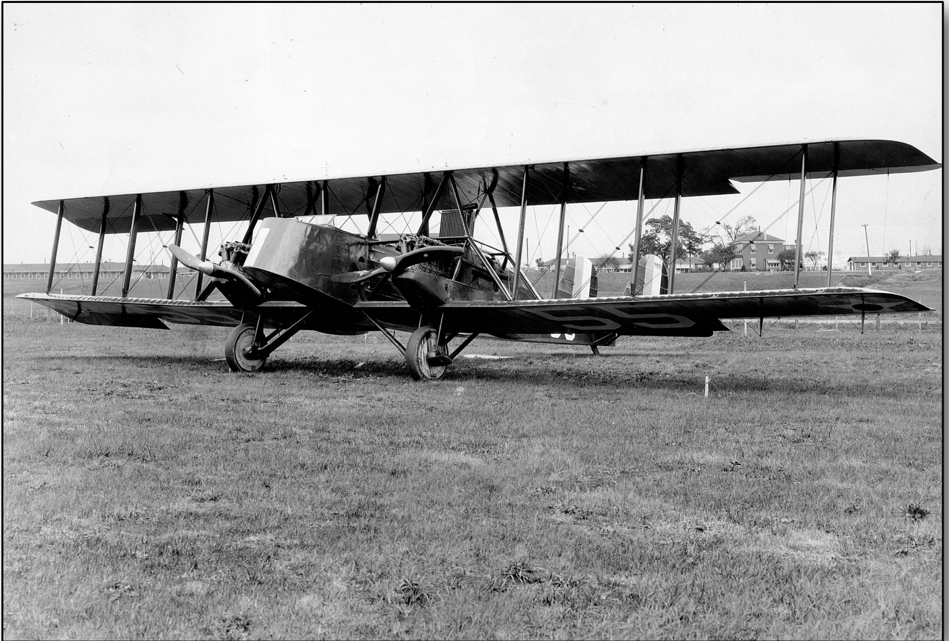
The Martin NBS-1 (MB-2) was the first U.S.-designed bomber, first ordered in June 1920 and replaced the British Handley-Page O-400 and Italian Caproni bombers in the United States from World War I. Derived from the MB-1, the MB-2 sacrificed speed and maneuverability to carry a heavy bomb load. The MB-2 became the Air Service's primary multi-engine bomber until it was replaced by the Keystone bombers in the late 1920s .
