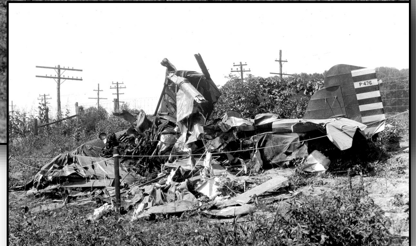
Top: Curtiss XO-1 Falcon pictured on 7 October 1927 with a Liberty engine. Right: Wreck of the Falcon on 4 September 1929, flown by Lt. George Schulgen, who was saved by his parachute, qualifying him for the caterpillar club. The crankshaft of the Liberty engine broke causing the propeller to fly off near Columbus, Ohio.
