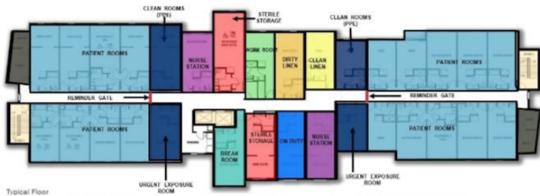
Figure 1. ACS Configuration with Individual Rooms
