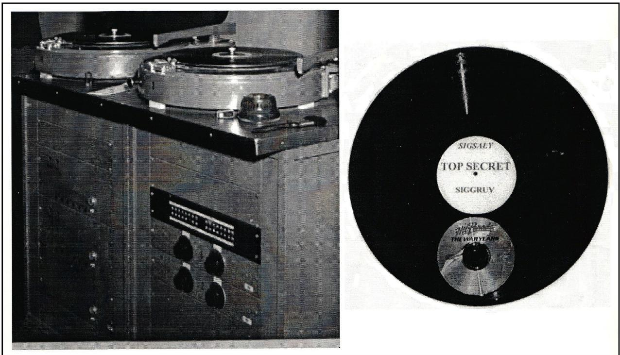
Fig. 10. A SIGSALY turntable and record, with a modern CD for scale<sup>20</sup>
