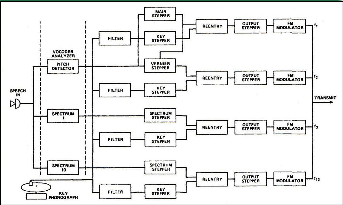
Fig. 9. An incredibly simplified schematic of a SIGSALY transmit terminal<sup>19</sup>
