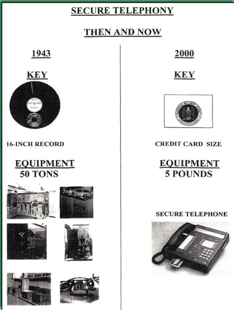
Fig. 19. A comparison between SIGSALY and a secure telephone from the year 2000<sup>35</sup>
