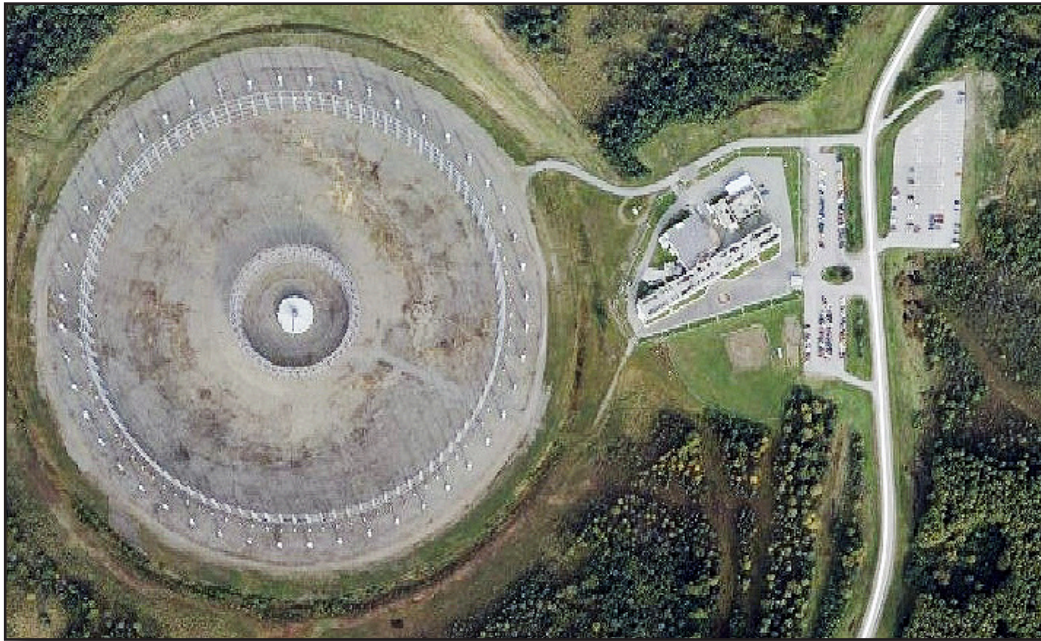
The AN/FLR-9 Wullenweber-class radio antenna, located adjacent to the 6981st Headquarters building on Elmendorf AFB.
