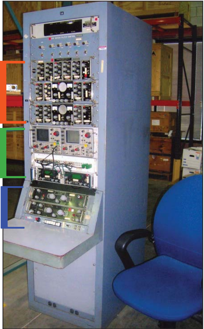
One signal collection “position” rack of equipment including the operator console and displays
