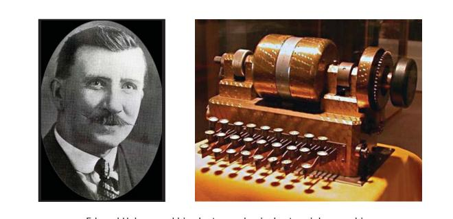
Edward Hebern and his electromechanical rotor cipher machine (courtesy of Ralph Simpson, CipherMachines.com)
