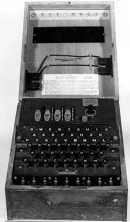
Figure 1 A four-rotor Enigma machine used by the German navy, the kind of machine Alan Turing was most concerned to solve.
