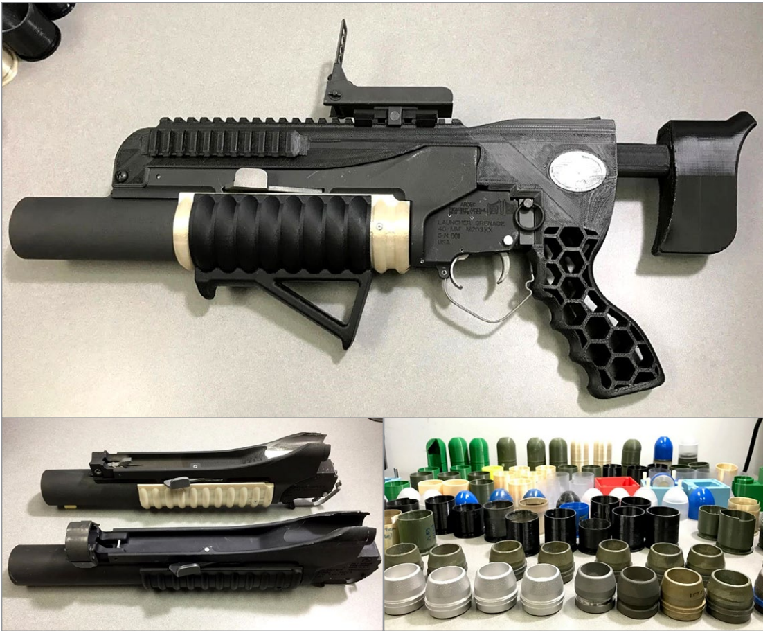
Figure 2. A 3-D Printed Grenade Launcher (Top), Grenade Launcher Parts (Bottom Left), and Miscellaneous Parts (Bottom Right) Source: The U.S. Army Armament, Research, Development, and Engineering Center.
