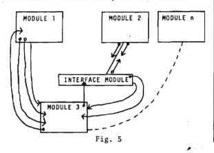
and 3 are unchanged. You are now in a position to redesign at your leisure module 1 and any other modules which invoke module 1. You can also deploy new modules which invoke module 3 through the interface without compromising their design because of deficiencies in module 3.
