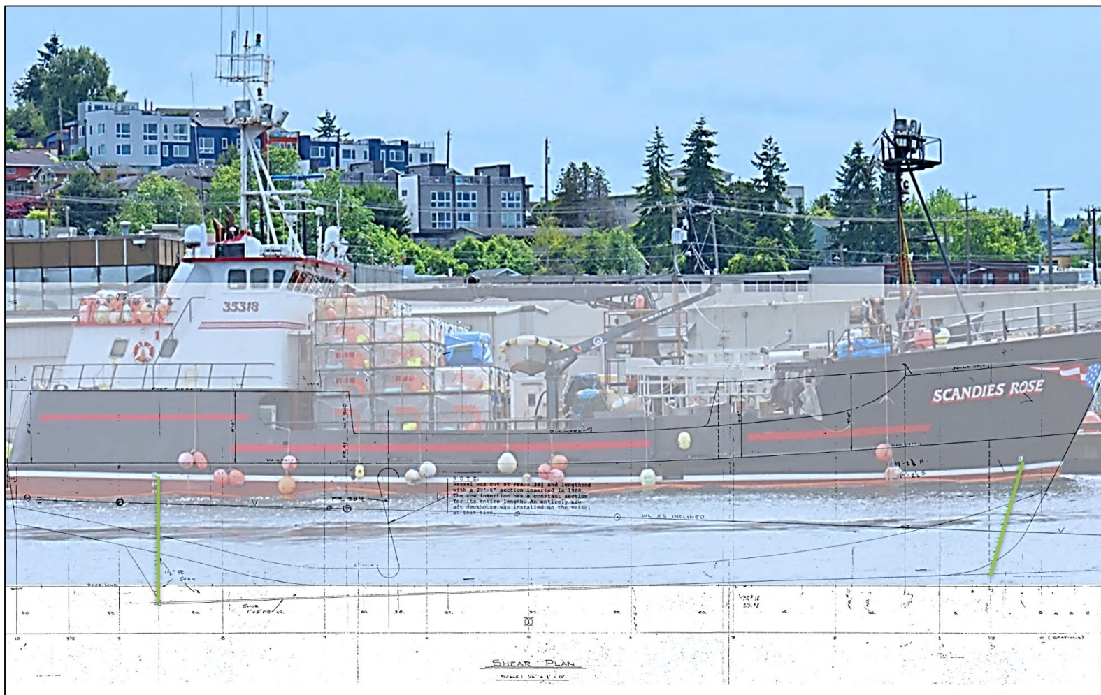
Figure 15: 2019 profile photograph from ref (o) with Lines Plan profile (ref (d)) and green draft marks overlaid to indicate MSC's assumed draft mark locations
