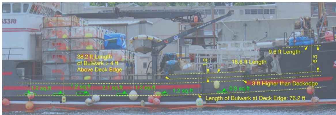
Figure 30: Profile Picture of SCANDIES ROSE from Ref (o) with Scaled Freeing Port Areas and Deck Lengths, the photograph and measurements are scaled with Rhinoceros drawing software
