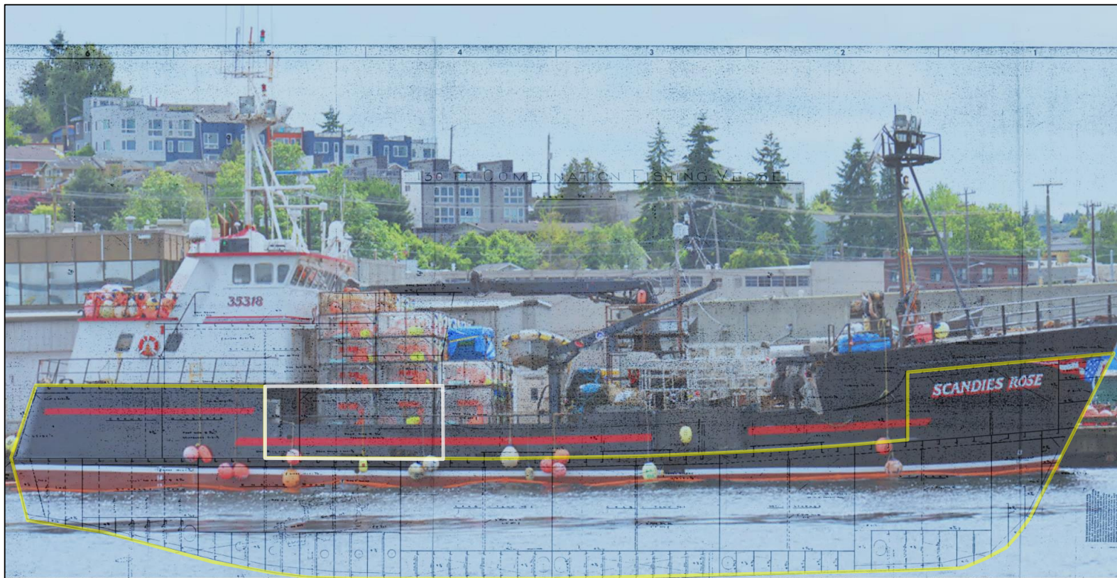
Figure 3: 2019 Profile photograph of SCANDIES ROSE from (ref (o)) with Scantling Plan and Profile (ref (e)) overlaid. Note that the plan matches the vessel's transom, but indicates additional buoyant volume at the forward end of the poop (white highlighted area)
