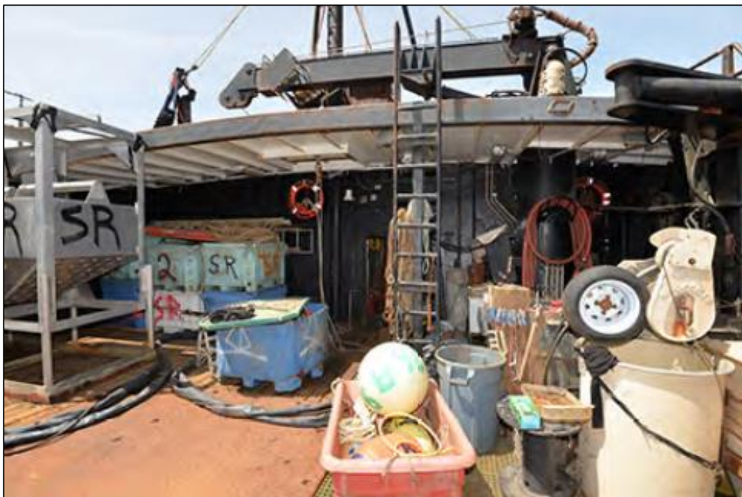
Figure 5: Photo from page 21 of ref (o) showing starboard crane pedestal aft of forecastle bulkhead
