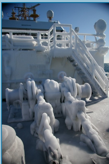
Ice accumulated on NOAA Ship Oscar Dyson Photo credits: NOAA Office of Marine and Aircraft Operations
