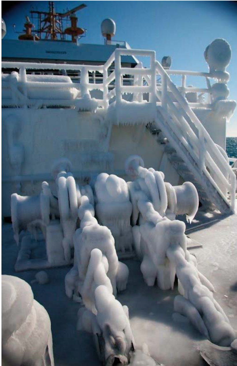
Ice accumulated on NOAA Ship OSCAR DYSON Photo credits: NOAA Office of Marine and Aircraft Operations
