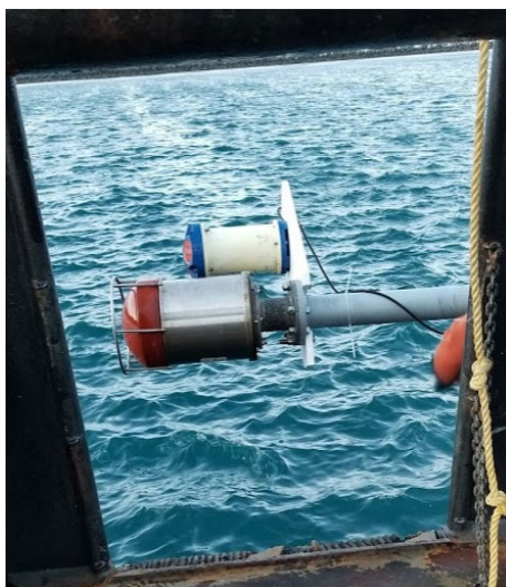
Figure 5 HiPAP (inboard) & ADCP (outboard) mounted on Endurance
