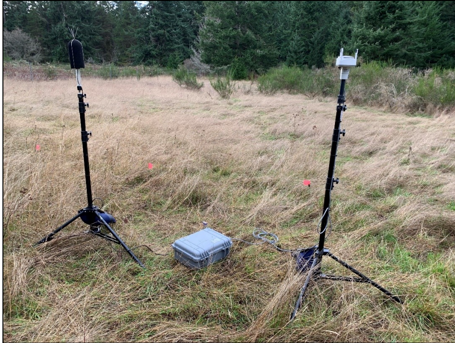
Figure 4.1 Sound Level Monitoring Station Deployed at NAS Whidbey Island (Site 8B_SG - Dog Park)
