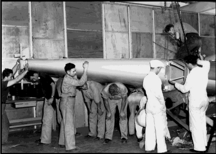
Sometimes brute strength and a strong back are required to get things done. Northrop technicians install the left main wing section of the N-1M.
