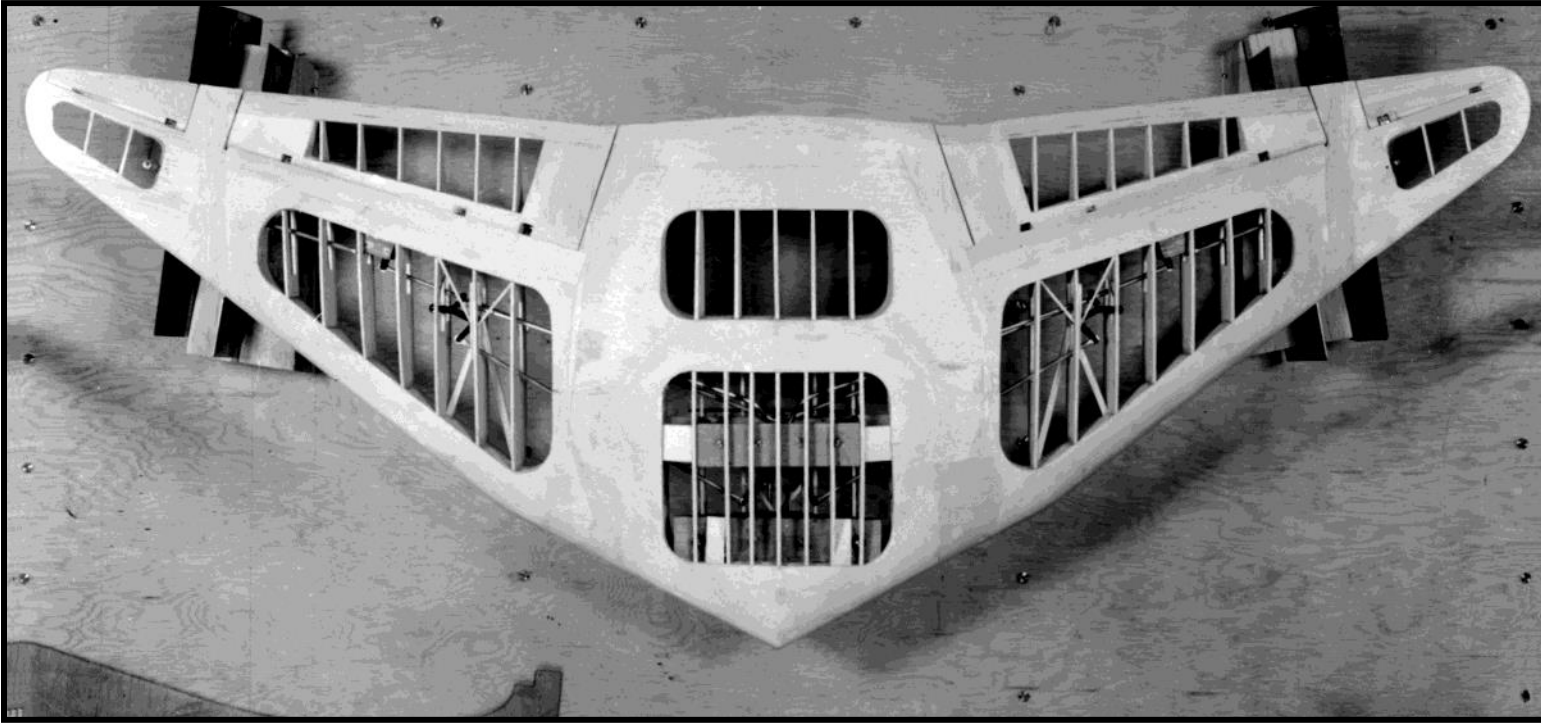
Northrop's talented craftsman built a variety of flying wing models including this one showing the basic internal construction of an N-1 design.
