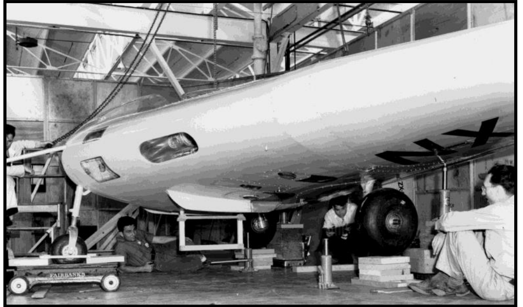
Weight and balance checks on the N-1M prior to taxi testing. Note the curved window panels in the nose. These would be covered over later in the test program.
