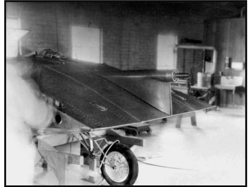
The swiveling, retractable aft landing gear and pusher propeller shaft installation show up well in this aft view of the Model 1's center fuselage.
