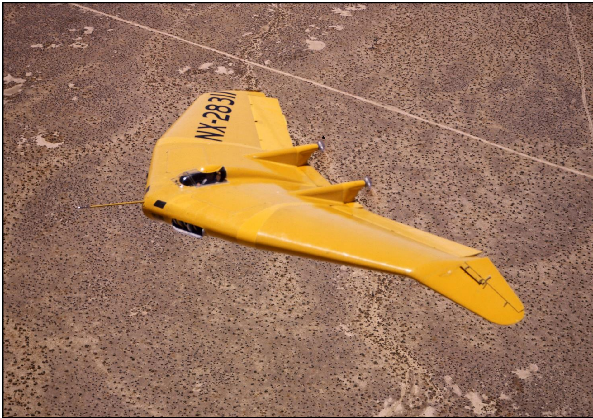
Although the N-1M had limited performance, it did prove Northrop's theory that an all-wing design was fully controllable. Data acquired from N-1M flight testing assisted in the design of the N-9M and XB-35 flying wing aircraft. Note the outer wing sections are adjusted aft a few degrees.
