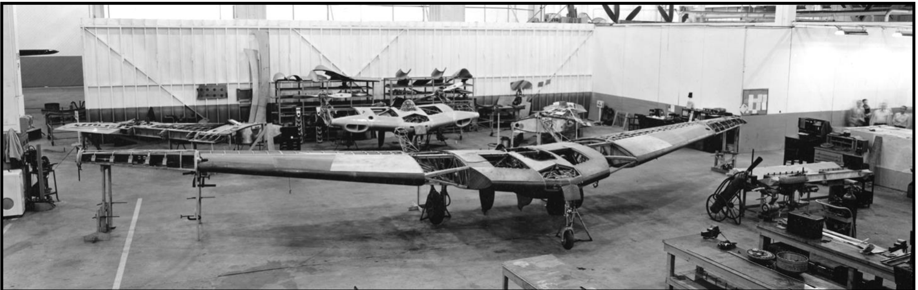
Two of the first three N-9M aircraft under construction at Northrop. A fourth airframe was added to the contract after the loss of the first airplane. Each airframe received its own designation; N-9M-1, N-9M-2, N-9MA and N-9MB.
