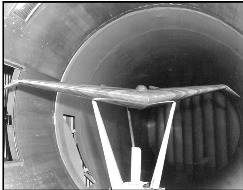
Wooden wind tunnel models of the N-1 design. The early design (above) shows large, fixed main wheels and tail skid, while the later design (right) is more refined with cockpit and engine shaft housings being added.
