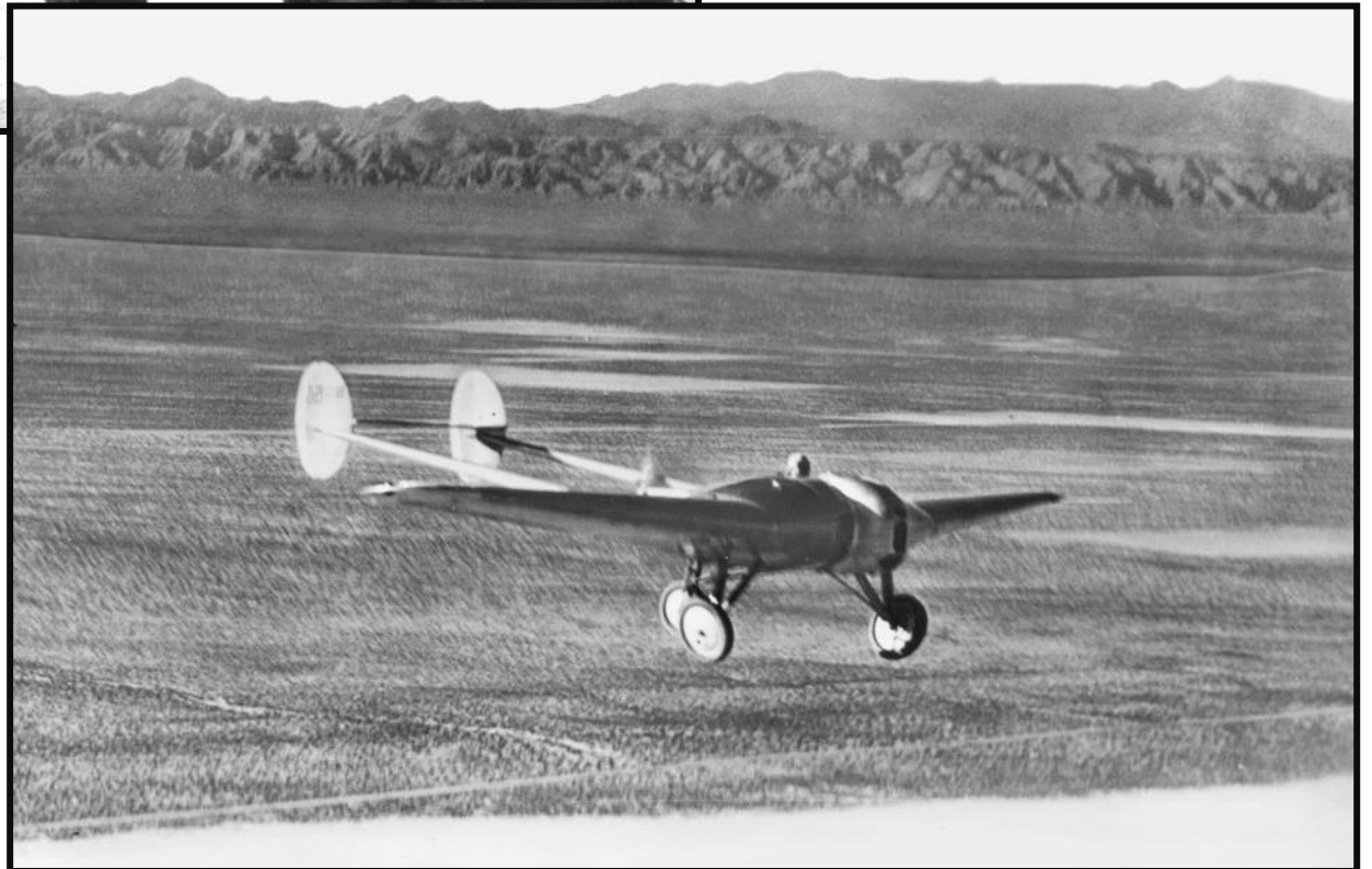
The Model 1 shown during a test flight near the Muroc Dry Lake test location. The retractable landing gear has been replaced by fixed gear.
