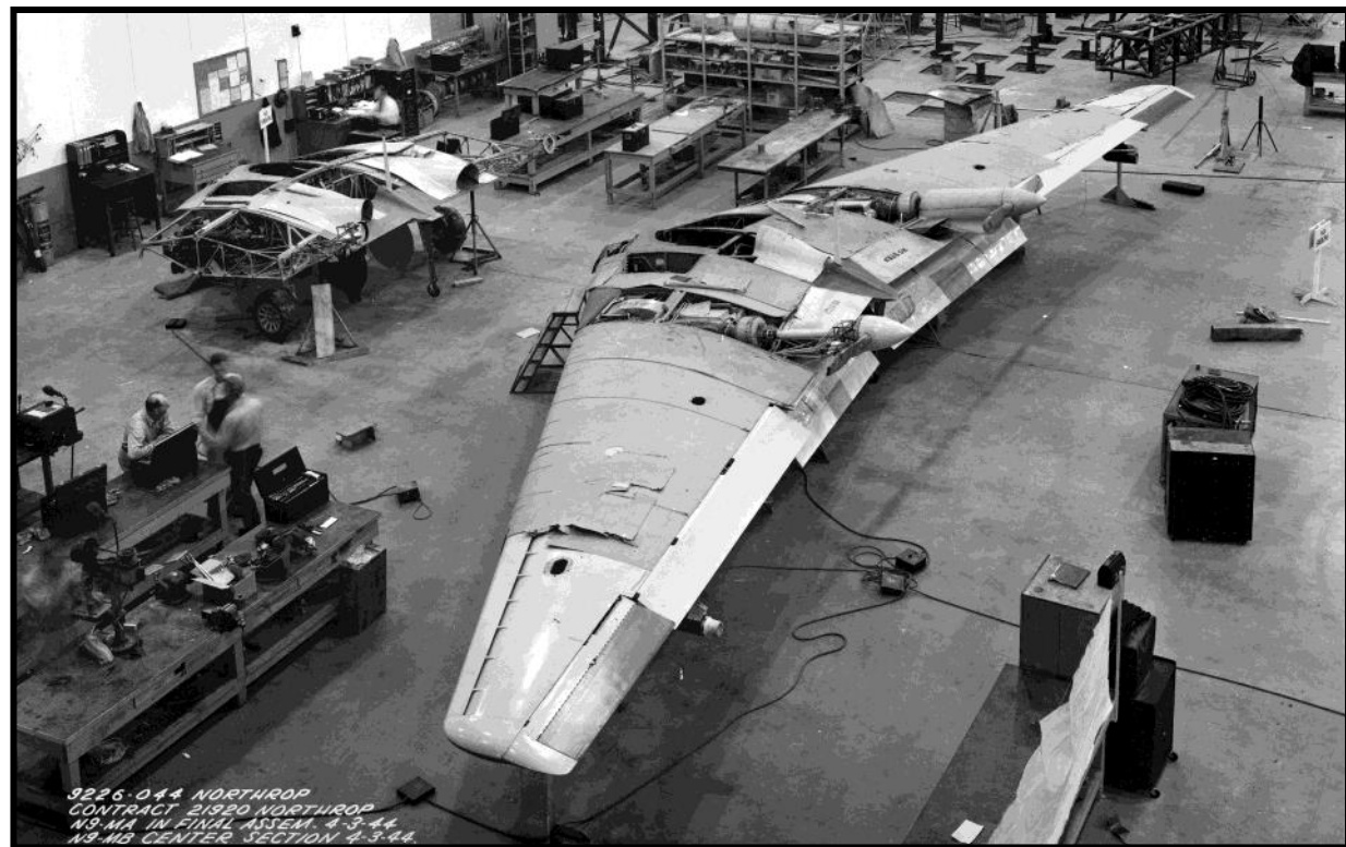
Center fuselage section of the N-9MA under construction at Northrop. The N-9MA used the same Menasco engines with a redesigned control system utilizing improvements learned from the first two aircraft.
