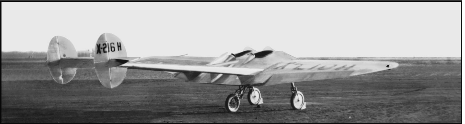
The Model 1 at Mines Field, Los Angeles, California shortly after final assembly at Avion Corporation. The two cockpits of the Model 1 show up well in these views. Both had windshields installed to protect the crew from the effects of wind, but later removed due to drag. Northrop pilot Edward 'Eddie' Bellande performed two short hops at Mines Field on July 30, 1929 prior to shipping the aircraft to Muroc Dry Lake for future flight testing.
