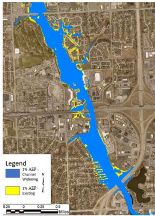
Figure 26 1% AEP Unsteady Flow Modeling Results for Channel Widening on the Big Papillion
