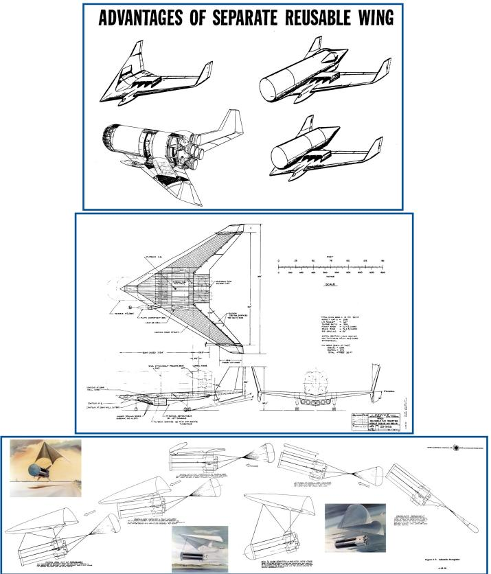
**All:** Significant research effort was put into making the Apollo Saturn boosters recoverable. The specialized, removable carrier aircraft designed by Boeing in 1963, could act as a first stage for the Saturn vehicle stack or utilized as a transport for outsized cargo. Paraglider recovery of a Saturn booster was also studied. Utilizing a Rogallo Wing parasail and retractable skids, the booster would glide down to a smooth recovery and refurbished for another mission.
