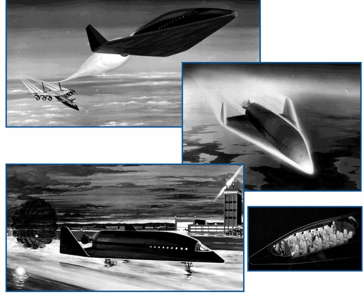
**Right and Below:** Under Air Force System Requirement (SR) 19786 for an Aerospaceplane, Douglas Aircraft proposed two different hydrogen -fueled single-stage-to-orbit (SSTO) designs. Both projected putting up to a 30,000 pound payload into a 100 to 300 mile earth orbit using a combination of reaction controls and large aerodynamic surfaces.
