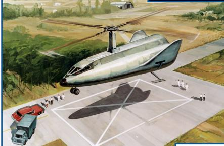
All: Some fanciful proposals utilized rotary wings for recovery. Proposals varied between designs, with some craft having the rotary wings stored internally while others stored against the exterior of the fuselage. This concept would be reborn in the late 1990's for the Roton Rotary Rocket which made only 3 hover flights in 1999 before being cancelled.
