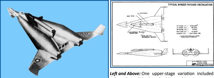
a Dyna-Soar glider launched into orbit using an expendable booster system that include a Minuteman first stage matched with an Thor-Ablestar second stage.
