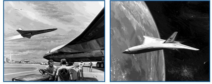
**Above:** The use of reusable launch systems is revisited in the 1970's by Rockwell International with their Star-raker concept. The HTOHL, single-stage-to-orbit design made use of 10 Mach 6-capable turbo-ramjet engines for atmospheric flight and 3 liquid-propellant rocket engines for orbital flight. Large for its time, the Star-raker had a 360 foot wingspan and payload capacity near 200,000 pounds.
