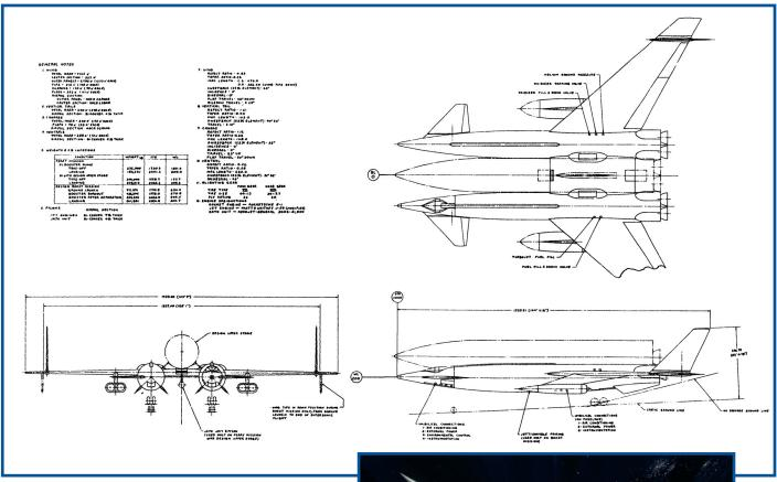
**Right:** This design from Lockheed made use of a large reusable first stage, an expendable second stage with a winged, orbital recoverable third stage. The concept, known as RAPT (Reusable Aerospace Passenger Transport) was similar in design to many of the early MX-2276 BoMi (Bomber Missile) concepts.
