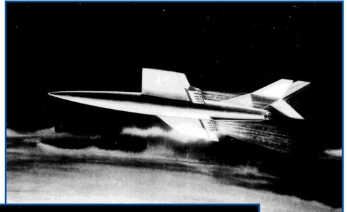
**Right:** The majority of space in this Douglas Aircraft design under SR-89774, stored propellants for the single nuclear engine capable of 817,000 pounds thrust. The structure of the 165 foot span wing would be made from titanium sandwich skin over a conventional aluminum frame. The small payload area in the front could be arranged to carry passengers or cargo. Note the skids used for main landing gear.
