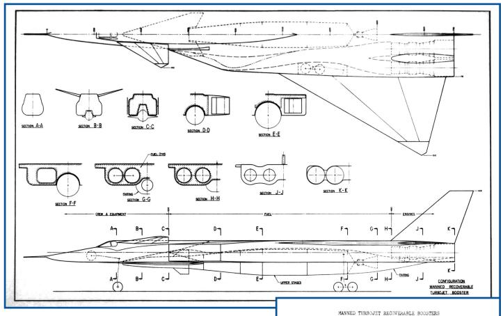
**Top:** North American Aviation proposed this unique design known as the Manned Turbojet Recoverable Booster using 4 Pratt & Whitney J91 nuclear powerplants to launch the expendable payload carried beneath the fuse-lage.
