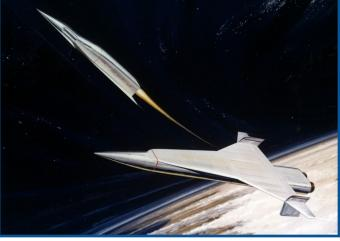
Right: The Boeing doublebody, winged booster, known as Model 832-40 made use of a Dyna-Soar glider as the crew module and escape capsule. Powered by twin clusters made up of 4 Rocketdyne J-2B rocket engines for vertical boost and 3 hydrogen-fueled, General Electric MF239C Turbofan engines for horizontal flight and landing. Designed for use with a variety of upper stages including this recoverable, delta-winged vehicle.
