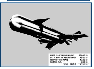
**Above:** Early designs from the Martin Company in 1961 took a basic approach to recovering the booster by simply adding fixed wings and a pair of airbreathing engines to the first stage. The same design process proposed similar modifications to the Titan II rocket to make it recoverable.
