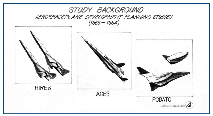
**Above:** Results from initial Aerospaceplane studies conducted by the Research and Technology Division, Air Force Systems Command, provided insight into the comparison of three different design concepts funded by the Air Force; Douglas Aircraft- Hypersonic In-flight Refueling Studies (HIRES); General Dynamics Astronautics- Air Collection and Enrichment System (ACES) and North American Aviation- Propellants On Board At Take Off (POBATO).
