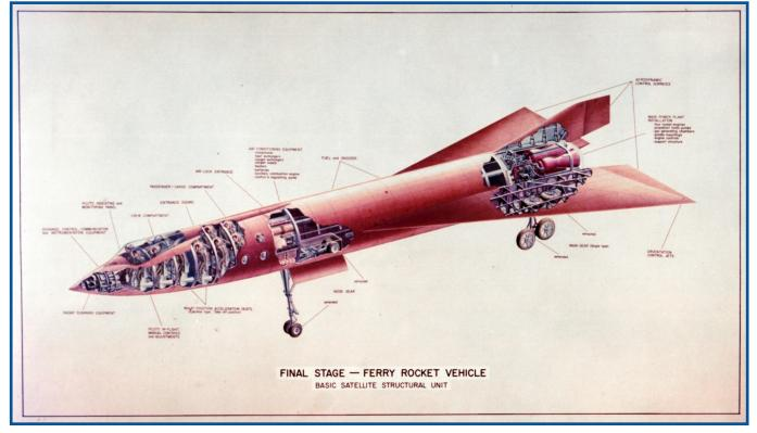
**All:** The ferry rocket of METEOR Jr. contained space for up to 14 passengers and crew, each placed in multi-position acceleration seats capable of ejection in case of emergency. The Air Force and NASA each funded studies at Goodyear based on the METEOR concepts, but never advanced beyond these studies. As shown below, the vehicles could be used individually or docked together as required by mission parameters.
