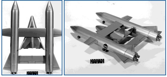
**Above:** This twin-boom design from NASA Langley Research Center carried a vehicle based on the HL-10 lifting body and was similar in design to the Martin Marietta Spacemaster. The twin-boom concept would make a comeback with the Scaled Composites Model 351 Stratolaunch vehicle, first flown in April 2019.
