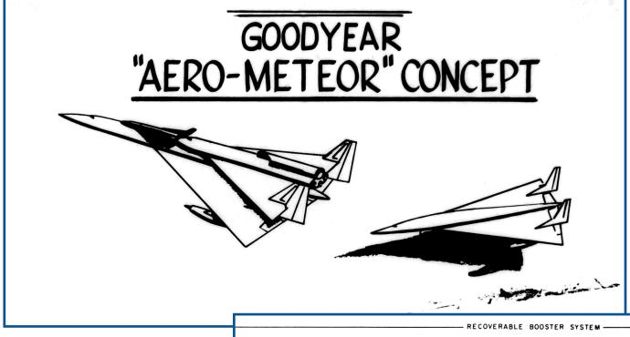
**All:** Goodyear Aerospace spent many years studying the use of recoverable booster systems. This later design, known as the Aero-Meteor made use of 3 winged vehicles to achieve orbital flight. The first stage used 6 hydrogen -powered, Pratt & Whitney (P&W) STRJ-84D turbo-ramjet engines, the second stage 2 Rocketdyne J-2 rockets plus a single turbo-ramjet engine and third stage utilized 2 P&W LR-115 rockets along with a single General Electric J85 turbojet for landing.
