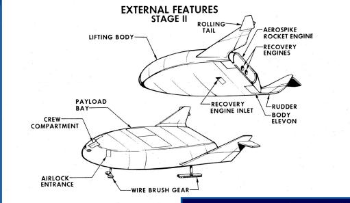
**All:** The POBATO second stage was of similar construction and included a moderate payload bay atop the vehicle. The wire brush landing skid system is noteworthy as is the use of aerospike rocket engines for main propulsion. Although the POBATO system was preferred over the ACES concept, the decision was made to place the entire Aerospaceplane project on the back burner until firm military space mission requirements had been defined.
