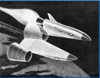
**Above:** One of Martin Company's Astrorocket proposals used an air-augmented rocket design known as a rocket engine nozzle ejector (RENE) to increase thrust of the booster vehicle.
