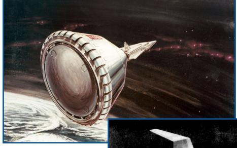
**Left:** The Chrysler SERV (Single-stage Earth-orbital Reusable Vehicle) proposed utilizing a twelve module LH2/LOX aerospike engine around the rim of the base, covered by movable shields. Two RL-10 rocket engines provided de-orbit thrust for this vertical takeoff and landing design. Note the lifting body spaceplane, MURP (Manned Upper-stage Reusable Payload), on top of SERV.
