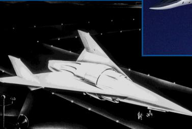
**All:** Manned hypersonic flight has long been a challenge for the aerospace industry. This proposal from Republic Aircraft made use of airbreathing scramjet engines around the center fuselage and proposed using the B-70 Valkyrie as a high-speed carrier vehicle. Note the design evolution from mid-wing to high-wing in the photos above and at right.
