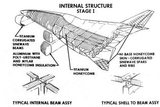
**All:** Under the Aerospaceplane Development Planning Studies program, North American received \$500,000 to study the POBATO (Propellants On Board At Take Off) concept. The two-stage POBATO made use of 8 turbo-ramjet engines on the modified lifting body first stage with the entire external structure made of metallic honeycomb sandwich material for reusability.
