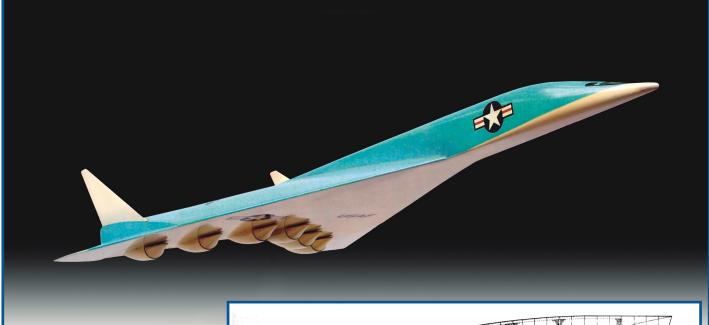
**Above:** Convair Versatile Spaceplane concept for the U.S. Air Force made use of six, large scramjet engines mounted under the wing.
