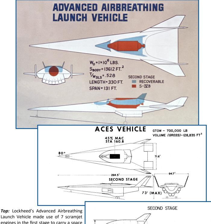
Launch Vehicle made use of 7 scramjet engines in the first stage to carry a space vehicle propelled by either a recoverable, winged second stage or an expendable S-IVB stage from the Saturn booster.
