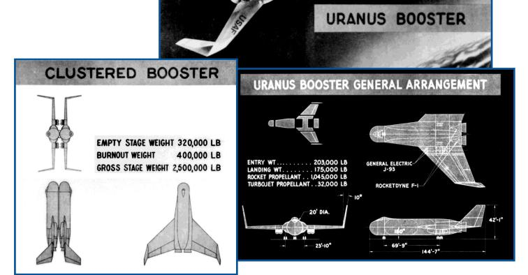
**Three above:** In 1961, Lockheed Sunnyvale proposed the universal recoverable booster system known as Uranus. With an empty weight of 160,000, the Uranus booster weighed less than a Boeing B-52 Stratofortress. Lockheed designed the vertically launched, horizontal landing vehicle around the use of 2 Rocketdyne F-1 rocket engines, but also provided alternatives using the less-capable E-1, plus 4 General Electric J93 airbreathing engines for horizontal flight and landing.
