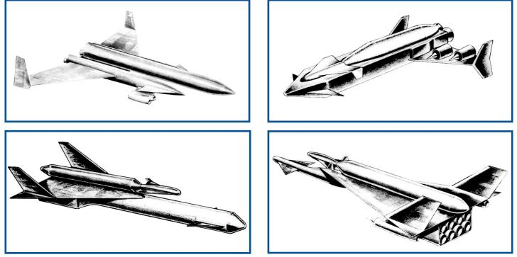
**Above:** Continued from page 6–clockwise from top left; VTOHL-Twin Fuselage-Parallel Staging; VTOHL-Three Stage-Hyperjet; Horizontal Takeoff and Landing (HTOL)-Three Stage-Turbo-ramjet; HTOL-Three Stage-Turbo-ramjet-JP-6 fuel (used specifically in the General Electric J93 engine).
