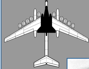
**Left:** One of many concepts proposed by Robert Salkeld of United Aircraft was this ten-engine monstrosity that carried a small, stage-and-a-half orbital craft. The small craft carried beneath the carrier ship would be boosted into orbit with the use of a liquid-fueled engine fed by external tanks located along the sides of the vehicle.
