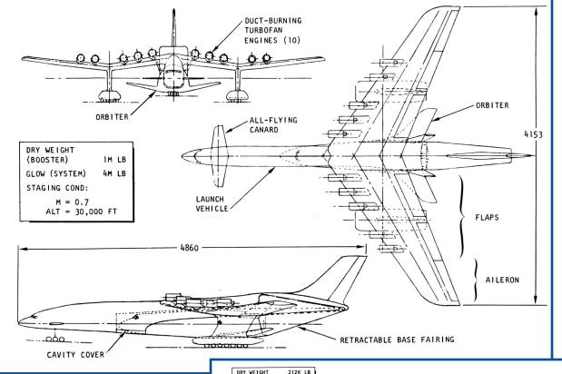
**All:** Rockwell's subsonic concept placed 10 duct-burning turbofan engines on top of the wing with the orbiter carried beneath. The subsonic carrier vehicle carried a larger orbital vehicle, powered by 2 RP-1-fueled rocket engines and 2 liquid hydrogen-powered engines, to an altitude of 30,000 feet and Mach 0.7 for release. All four engines on the orbiter firing simultaneously at launch to propel the orbiter into space.
