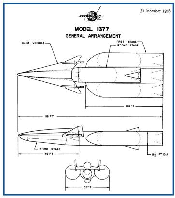
**Above and Right:** The Douglas Model 1377 began as a 6 month study under project RoBo (Rocket Bomber) with an expendable first and second stage and only the glider being reusable. By June of the following year it evolved into having a reusable, airbreathing first stage. The glider's design used Inconel X as the primary structure and is unique in having the pilot in the rear of the vehicle.
