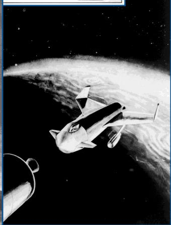
**All:** This North American Aviation (NAA) recoverable booster design began as a proposed booster for Boeing's Dyna-Soar. Boeing subcontracted NAA for a series of studies on a recoverable booster. The Rocketdyne F-1-powered design was also proposed as a crewed vehicle with the addition of a crew compartment and canards on the forward structure.
