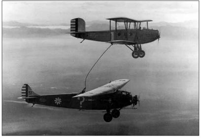
The first sustained test of air refueling occurred in 1929 when the flight of the *Question Mark* stayed airborne for more than 150 hours across 43 in-flight refuelings. Note the hose being held by an occupant of the receiving aircraft, possibly Maj. Carl Spatz (the spelling later changed to Spaatz).
