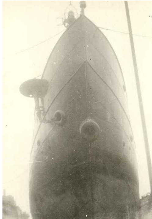
"[From the top of the forward stick, this is the] view of bow from forward stick." Note the spare mushroom anchor secured to starboard.
