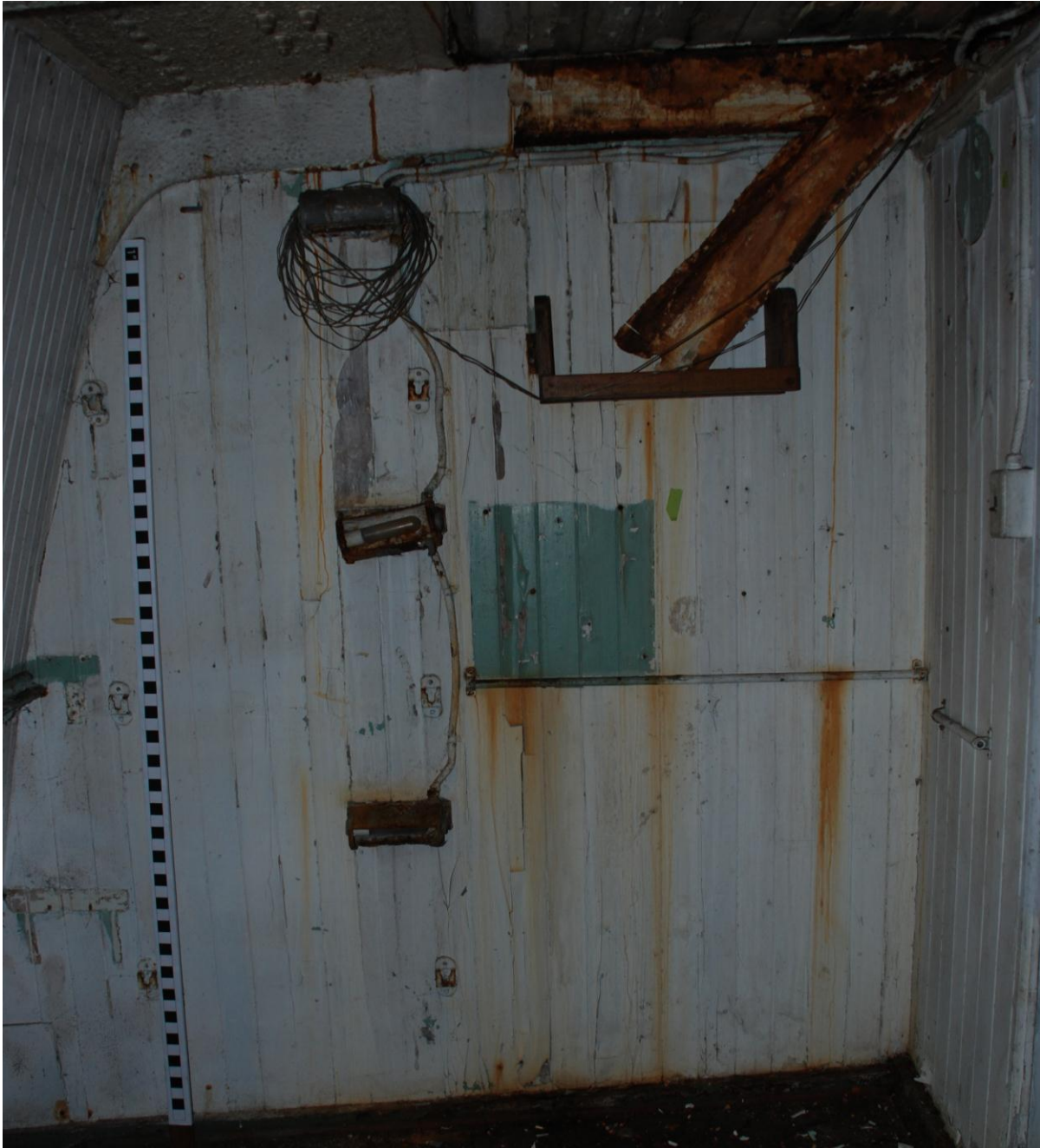
FIGURE 51. Port Side Crew Quarters. Three bunks were removed from the inboard partition. Ghosting and light fixtures allow for a visual recreation of how the cabin would have looked while inhabited by crew. Note the various shades of paint as well as deterioration. Scale is 1 inch. (Photo by author, 2010.)
