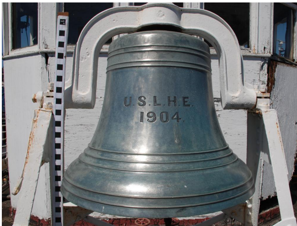
FIGURE 39. This is the 1,000 pound, metal signaling bell installed onboard LV83. Scale is in inches. (Photo by author, 2010.)
