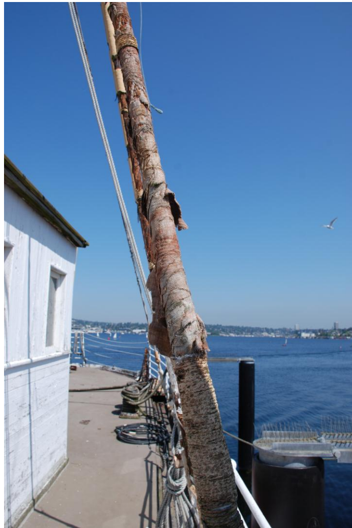
FIGURE 47. Different wrapping techniques on shrouds. Note the change in wrapping width from 1.25 in., to 2.25 in. (Photo author, 2010.)
