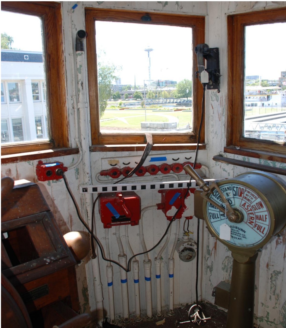
FIGURE 48. Pilot house communication switches, wiring, and devices. Note that wires traveling between decks are protected by metal tubing. The phone and phone cord plugged into the communications outlet indicates how devices were connected to the onboard system. Similar outlets installed throughout the ship enabled communication with the bridge at all times (Photo by author, 2010).
