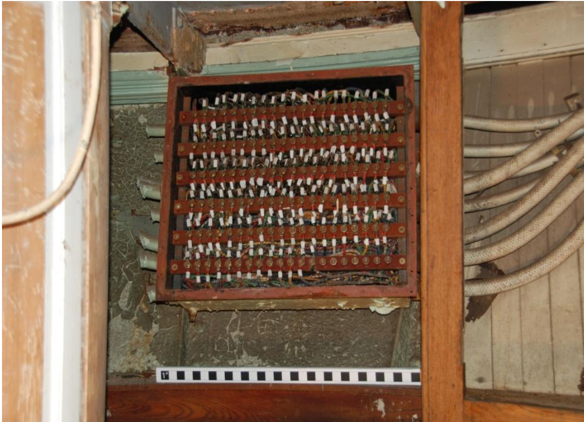
FIGURE 8. Degaussing coils onboard LV83. Photo shows the main distribution panel and coils. The coils on the starboard side have been severed but are intact on the port side. Scale bar is in inches. (Photo courtesy of the author, 2010.)
