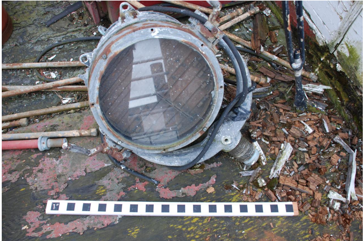
FIGURE 46. A signal light on the weather deck of LV83 . This artifact was photographed with a scale bar and tagged with an accession form indicating found location, present condition, and accession number. (Photo by author, 2010.)
