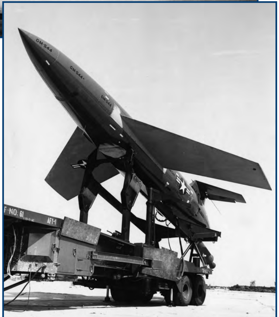
Top and Bottom: With initial test launches performed from a concrete hard stand at the Missile Test Center, latter launches made use of a specially designed mobile platform.
