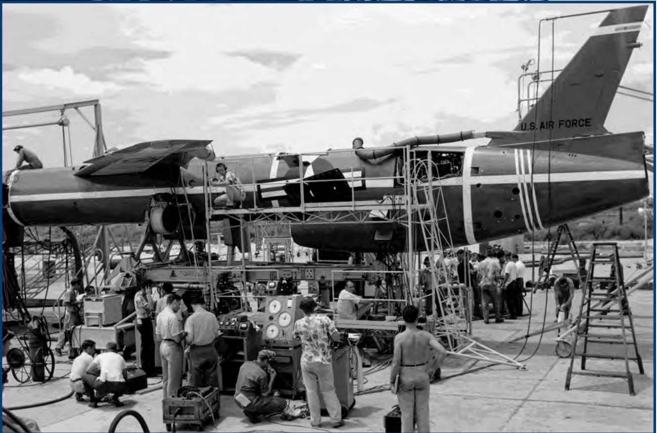
All: The early N-69 missiles were labor intensive to prepare for launch. A number of specialized technicians required for the warhead, avionics, powerplant, navigation and other systems of the Snark .
