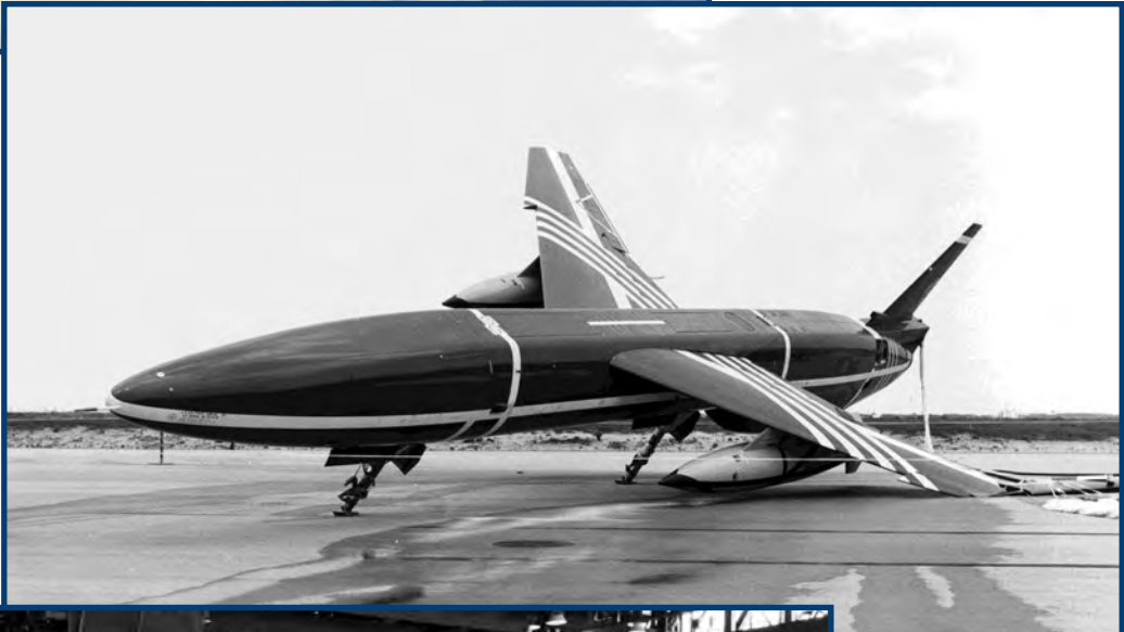
Right: Landing a Snark safely at the Skid Strip could be a challenging affair as shown in this photo taken April 16, 1957. Despite the damage to the left wing, this missile was repaired and flown again.
