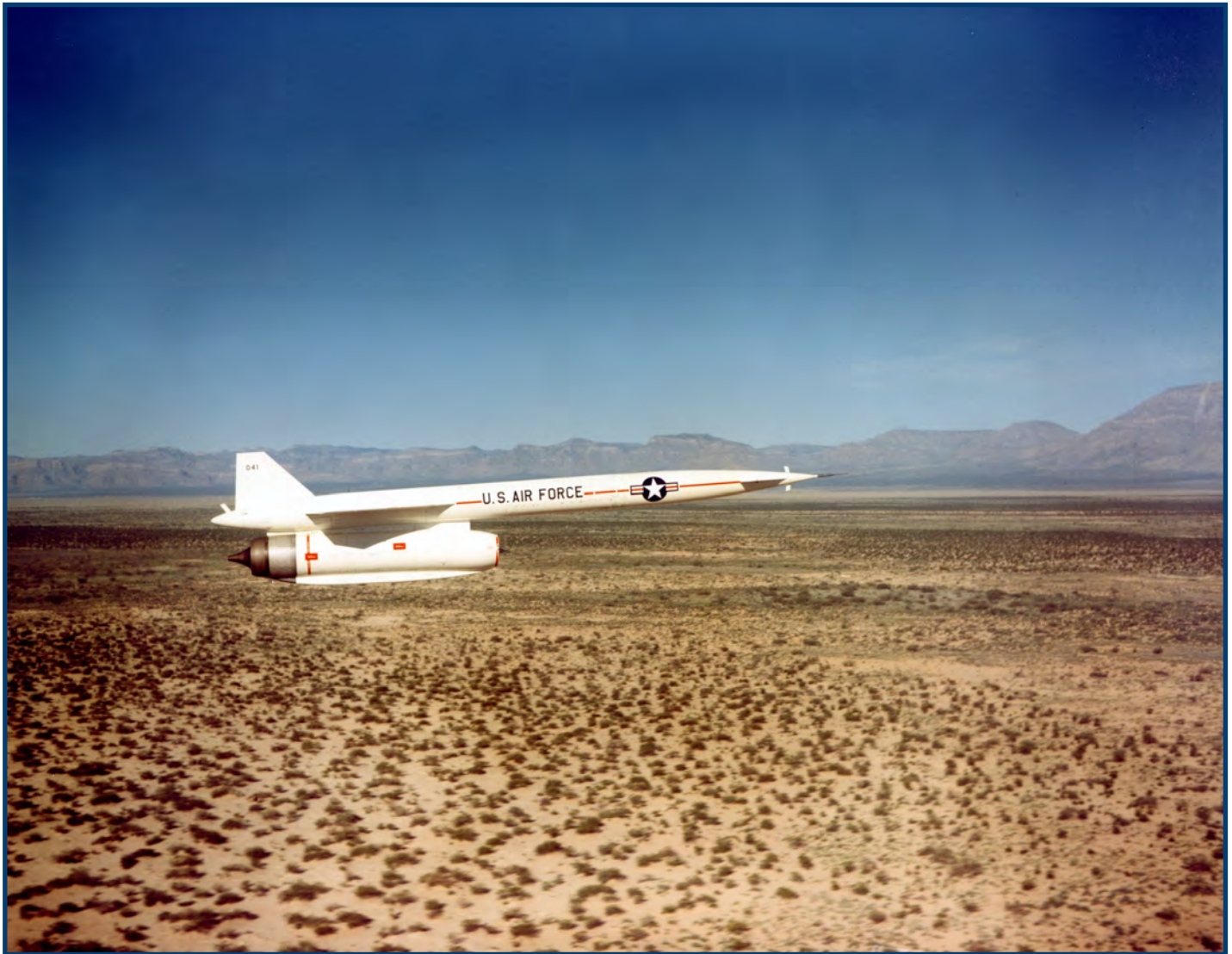
Above: GAM-77 Hound Dog cruises over White Sands Missile Range, NM. Depending on the mission, missiles could fly as low as 200 feet or as high as 56,000 feet.
