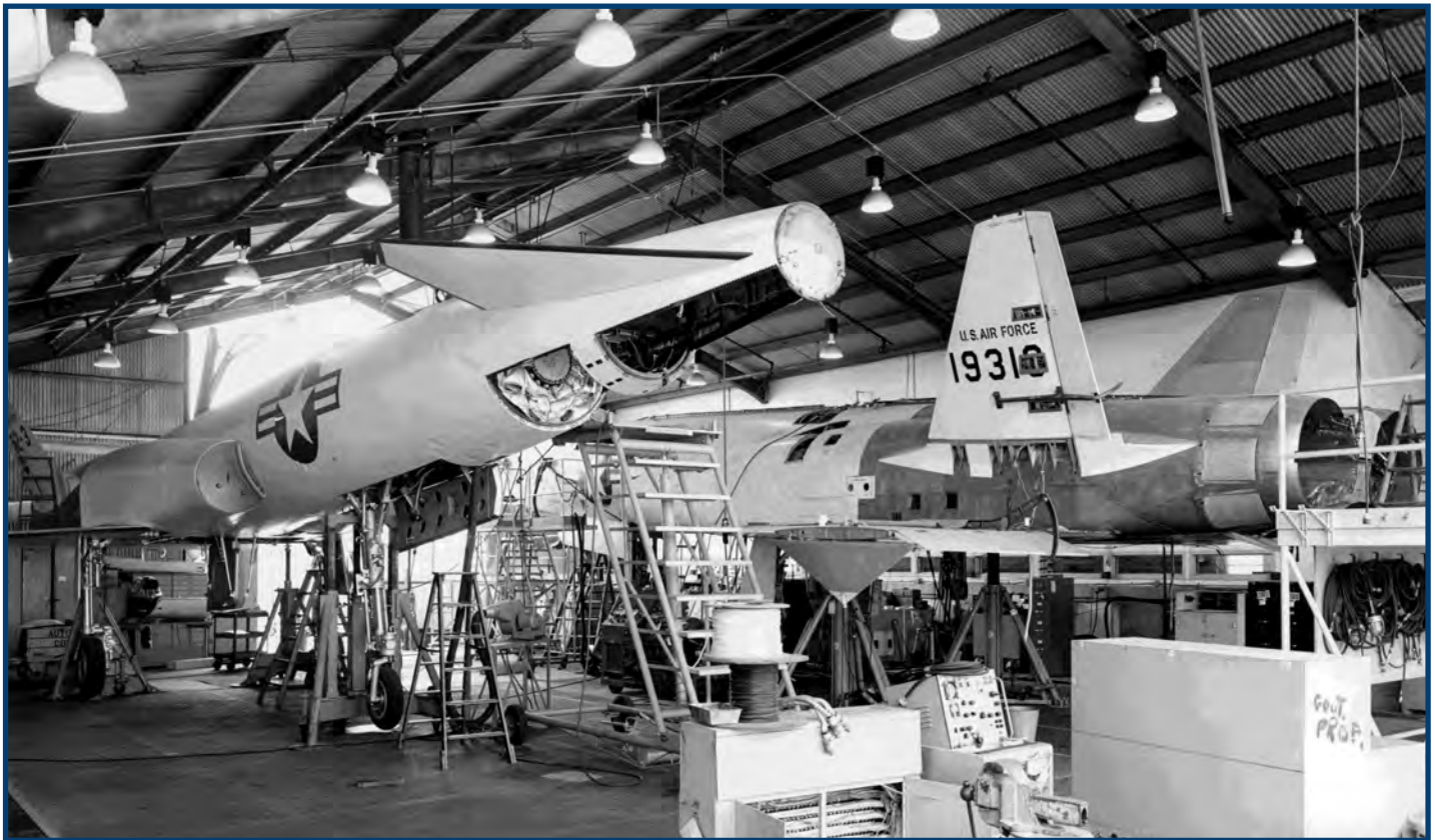
Above: The last two flyable X-10 missiles undergo modifications to become target drones for the BOMARC missile program.
