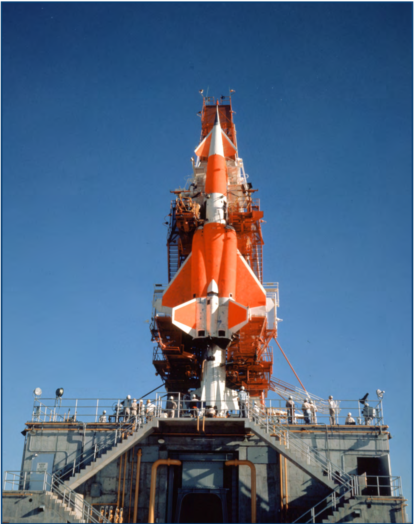
Above: Many of the XB-64 Navaho missile test vehicles were painted in bright color schemes to aid in long range tracking over the Atlantic Missile Range.
