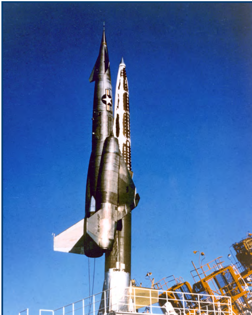
Left and Above: The second, and last, flight of a Navaho for Project RISE ended in failure when the vehicle broke up at 77,000 feet.
