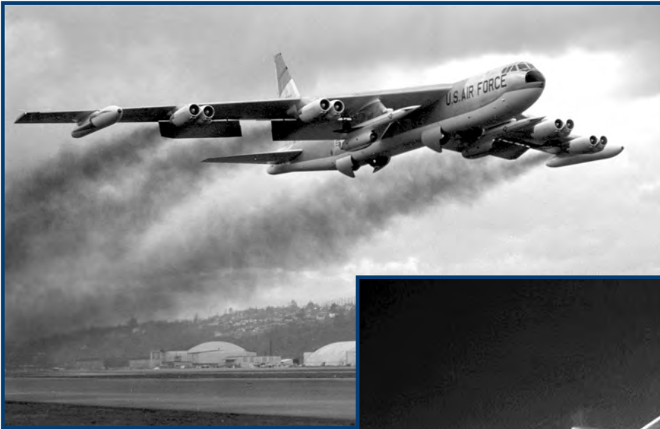
Left: With smoke billowing from the eight, water-injected Pratt & Whitney J57-P-43WA engines, this B-52F with two AGM-128 Hound Dog missiles departs its base to remain on airborne alert.
