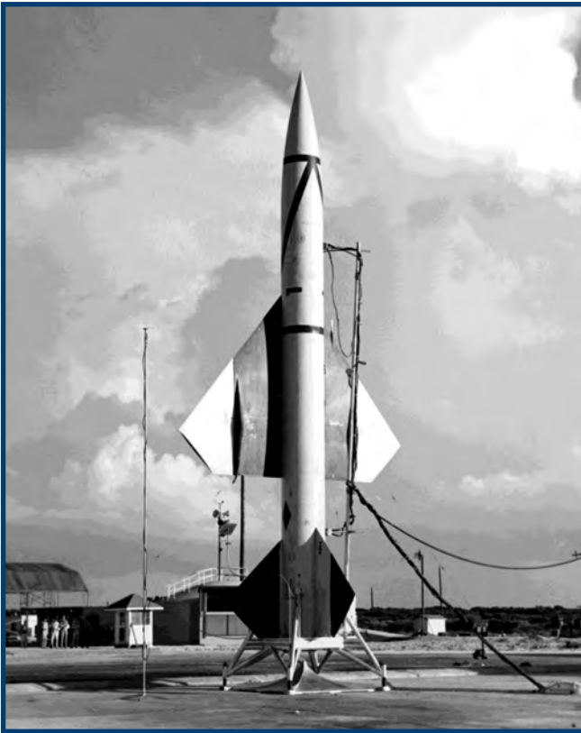
Top: First flown in 1952, the Boeing BOMARC ( BO eing Mi chigan A erospace R esearch C enter) originally carried an F-99 designation, but this changed three years later to IM-99. The XF-99 shown above had the vertical stabilizer on the bottom and did not yet incorporate the ramjet engines for cruise flight.
