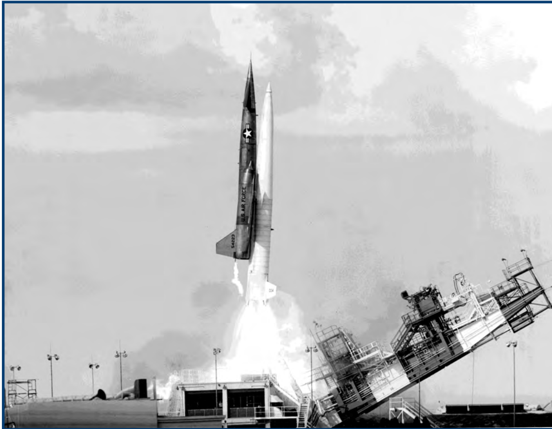
Left: With the red & white launch gantry moved out of the way, XB-64 Navaho , 55-4223, departs on the next to last flight during a Project RISE mission. This mission ended in failure when a fuel system malfunction prevented ramjet ignition.
