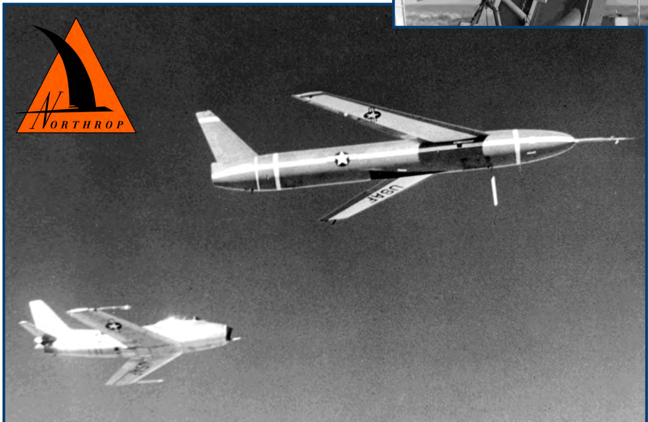
Above: Flight testing of the N-25 Snark took place over the White Sands missile test range after launching from Holloman AFB, New Mexico. Twenty-five flights with sixteen missiles reaching a max speed of Mach 0.9 with a max flight duration of 2 hours and 46 minutes.
