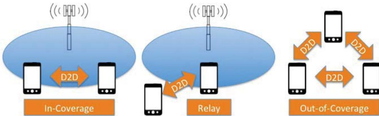
**FIGURE 4.** LTE Release 12 D2D use cases.
