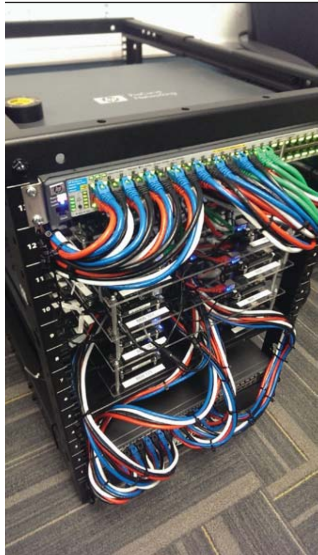
FIGURE 2. This RCPS test bed contains 32 embedded Linux computing boards. Each board (middle) is connected to both a smart network switch (top) which performs network emulation using OpenFlow and a regular network switch (bottom) that provides access to the physics simulation (Orbiter Space Flight Simulator).
