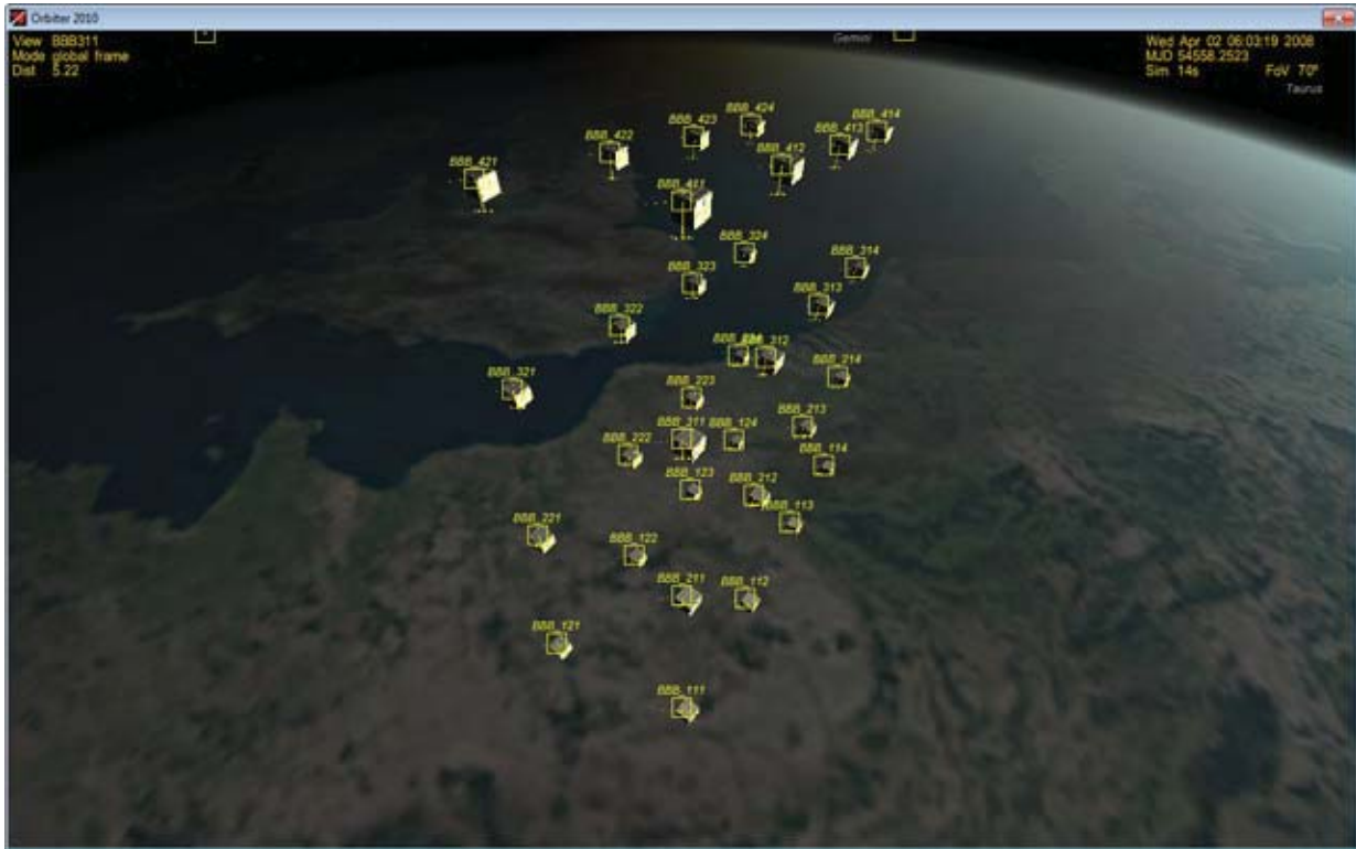
FIGURE 3. This Orbiter Space Flight Simulator simulation of the 32-node satellite cluster, which is controlled by the RCPS test bed, calculates the physics of the satellites and simulates their sensors and actuators.
