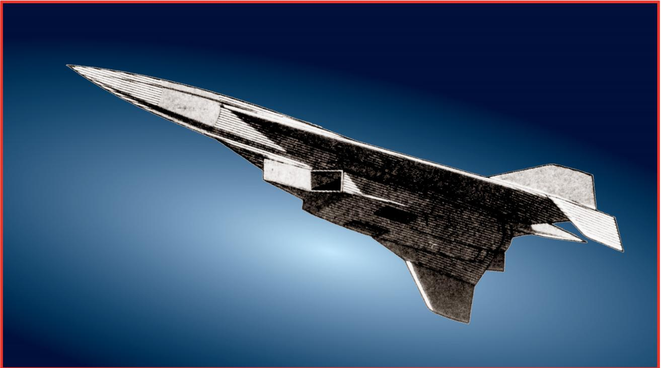
**Above:** One of the earliest design proposals to come out of the B-70 program is this October 1959 concept for a Recoverable Booster Support System (RBSS). Whether manned or unmanned, passenger or cargo carrier, launch vehicle or nuclear bomber, the B-70 Valkyrie design inspired the imagination of engineers and designers across all of the aerospace industry during the 1960's.
