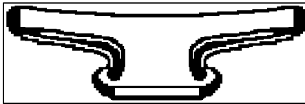
Figure 4-4: Welded Horn Type Deck Cleat
