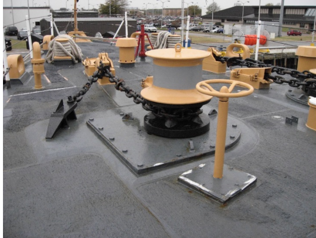
Figure 4-3: Vertical Shaft Windlass
