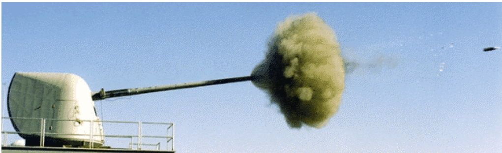
Figure 3.0-12: Gun Blast and Projectile from a 5-in./54 Navy Gun
