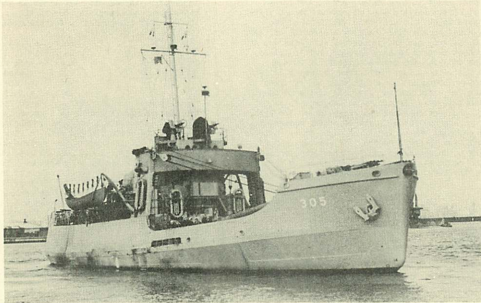
ICE BREAKER AND BUOY TENDER MESQUITE THIS COAST GUARD VESSEL IS A DUAL-PURPOSE CRAFT DESIGNED FOR ICE-BREAKING AND FOR BUOY TENDING
