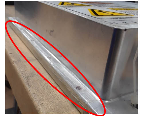
Missing security tape
