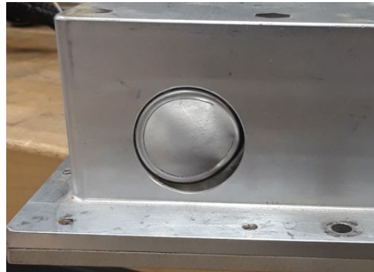
Damaged pressure vent
