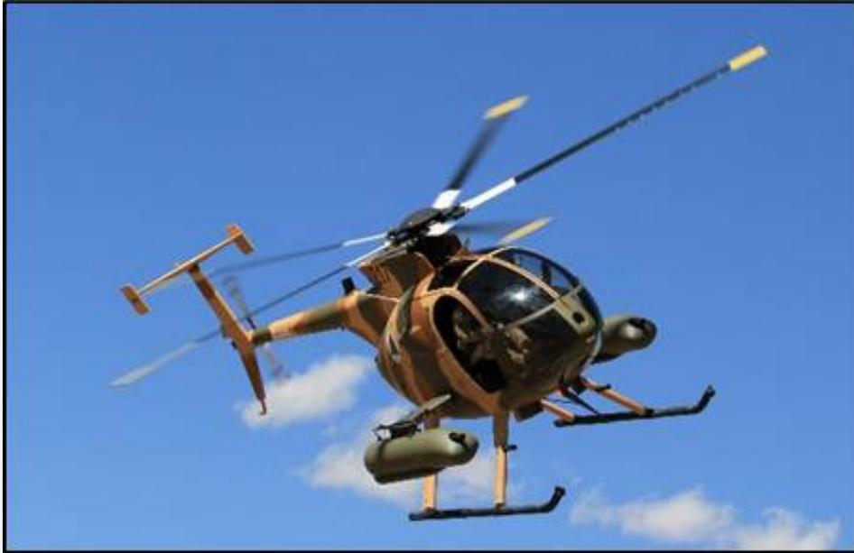
The MD-530 helicopter provides close-air attack and aerial escort to ground forces. The MD-530 has two weapons pylons with .50 caliber machine guns and rockets. As of October 26, 2019, the Kandahar Air Wing has three operational MD-530 Scout Weapons Teams.
