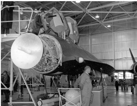
The Hughes ASG-18 was the most powerful aircraft radar system built at the time and a variant was eventually used in the F-14 Tomcat as the AWG-9/Phoenix missile system. (AFTC/HO)
