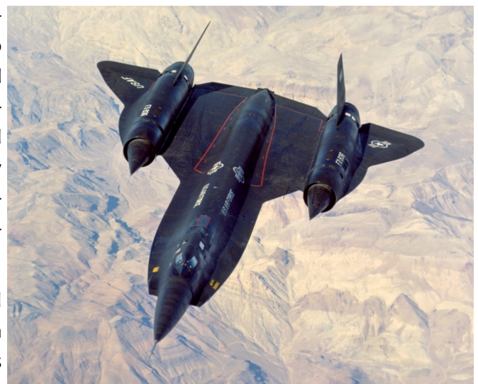
The nose chine and radome modification show up well in this view of a Lockheed YF-12A pulling up to the KC-135 tanker high over the Mojave Desert. (AFTC/HO)
