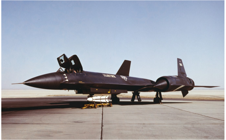
A Hughes AIM-47 missile sits next to the third Lockheed YF-12A Blackbird at Edwards AFB. The white silhouettes on the forward fuselage denote the speed and altitude records set in May 1965. (AFTC/HO photo)
