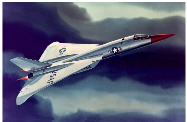
The North American F-108A Rapier would be powered by two General Electric J93 engines similar to those used in the XB-70 bomber. (National Archives, St. Louis)
