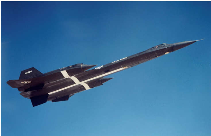
The third YF-12A departs Edwards AFB in 1965. The white cross painted on the lower fuselage assisted in tracking the aircraft during the speed and altitude record flights. (Lockheed photo)
