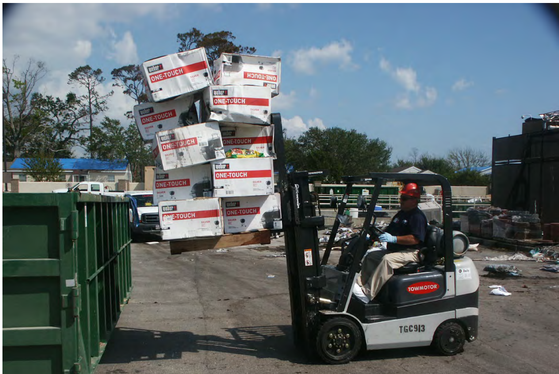
A worker uses a forklift to load flood-damaged merchandise from the Base Exchange at Keesler AFB into a roll-off for disposal at a Subtitle C landfill.
