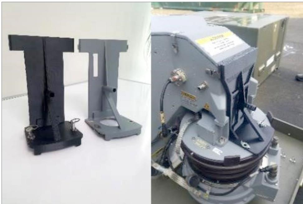
Figure 4. Traditionally Manufactured and AM-Produced MH-60R Airborne Low Frequency Sonar Covers
