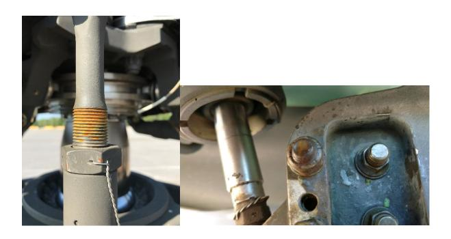
Preventable surface corrosion located on fully mission capable (FMC) aircraft. These aircraft were on the flight line ready to conduct daily operations. (Both pictures are of AH-64D/E common components)
