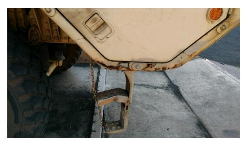
Heavy Expanded Mobility Tactical Truck (M977 HEMTT) with surface and penetrating corrosion on step and cabin frame. The vehicle was located on an undisclosed flight line ready to pump fuel into aircraft.
