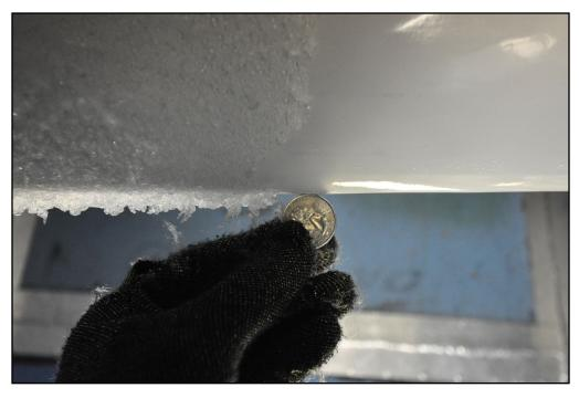
Leading edge of RQ-4 aircraft wing surface with and without using an active ice protection system. (photo courtesy of Battelle)
