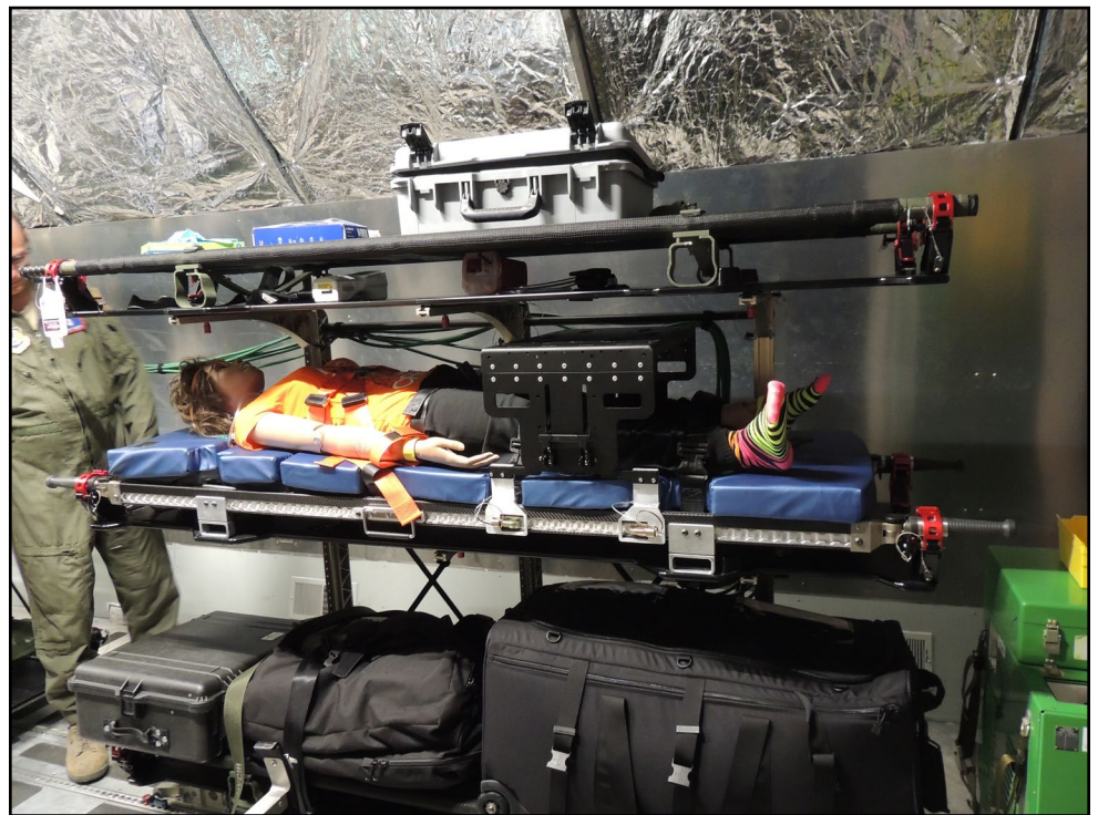
Cornerstone Research Group's aeromedical evacuation stretcher is shown during a compatibility test on a KC-135. (Photo courtesy of Cornerstone Research Group)
