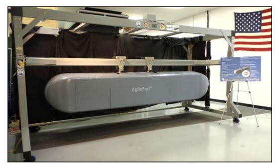
Air Force Research Laboratory's AgilePod is a multi-intelligence, open architecture, reconfigurable prototype designed for the intelligence, surveillance and reconnaissance (ISR) and Air Force Special Operations communities. The reconfigurable pod enables operators to customize sensor packages based on specific mission needs, enhancing the intelligence process. (Photo by Marisa Novobilski-Alia.)
