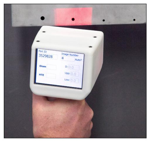
The Hole-to-Edge Measurement Technology system performs a non-contact inspection. The HEMT was developed by Creare, LLC under an Air Force Small Business Innovation Research agreement. The technology and other equipment was temporarily transferred to Creare, LLC under a Cooperative Research and Development Agreement with the Air Force Research Laboratory Materials and Manufacturing Directorate. (Photo courtesy of Creare, LLC.)
